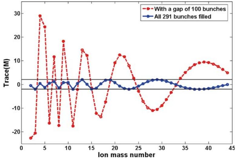
**Figure 2.** Trace of the transfer matrix of ion motion as a function of different ion species of mass upto 44[CO<sub>2</sub>] for all filled 291 bunches (blue solid curve) and for a gap size of 100 consecutive bunches (red dash curve). Stable zone is between the two horizontal straight lines.
