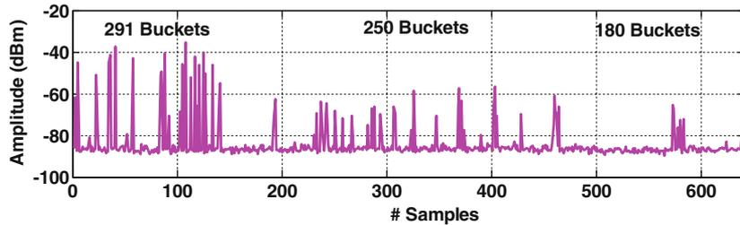
**Figure 8.** Amplitude variation of transverse coupled bunch instability in the vertical plane for different bunch filling patterns in Indus-2.
