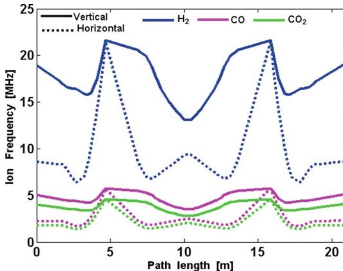
**Figure 3.** Variation of oscillation frequency of different ion species in both horizontal and vertical planes along the Indus-2 ring for one superperiod.
