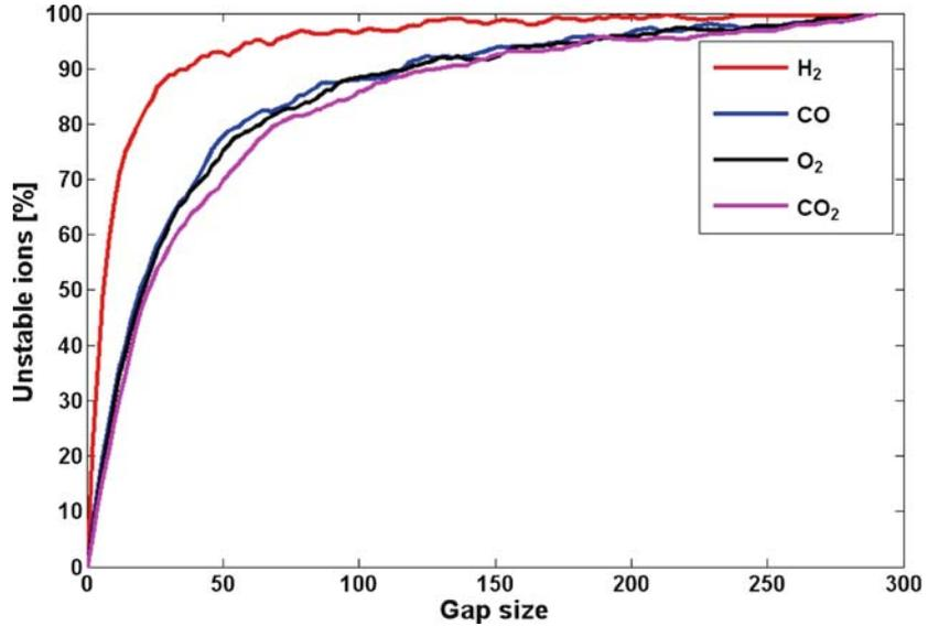
**Figure 5.** Percentage of unstable ions of various species for beam current up to 300 mA as a function of bunch gap size at 550 MeV in Indus-2.
