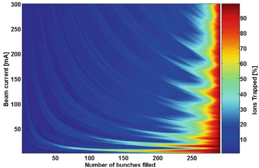
**Figure 6.** Region of ring circumference in percentage where the CO ions are trapped for different lengths of bunch train in the Indus-2 storage ring. The maximum length of the bunch train is 291.
