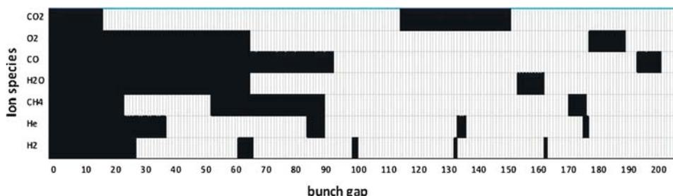
**Figure 4.** Stability of various ion species for different bunch gap sizes in Indus-2. Dark areas indicate the stability of ions.
