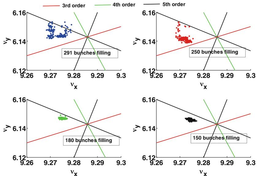
Figure 7. Variation of betatron tunes in both horizontal and vertical planes are illustrated in tune space for different bunch filling patterns in Indus-2.
