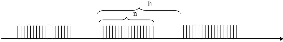
**Figure 1.** An illustration of the bunch train that shows a maximum possible  $h$  bunches out of which  $n$  bunches are filled with electrons and  $h - n$  bunches are empty.
