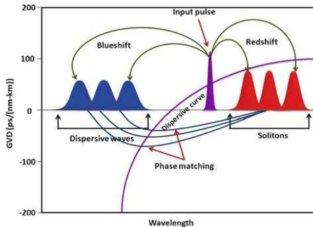
**Figure 5.** Scheme of a SCG by fission of higher-order solitons. Thick violet line is GVD for a PCF. Spectra of NSR, solitons and input pulse are presented by blue, red and violet colour pulses, respectively. The phase mismatch between solitons and NSR is presented by blue lines.
