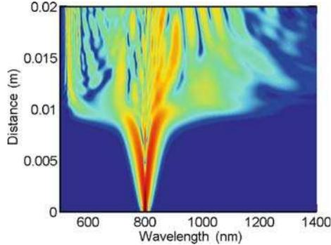
**Figure 6.** The SCG for 20 fs input pulse width in silica core PCF at 800 nm. The fibre parameters are  $\beta_2 = -0.0148883 \text{ ps}^2/\text{m}$ ,  $\beta_3 = 0.000032771 \text{ ps}^3/\text{m}$  and  $\beta_4 = 1.19 \times 10^{-7} \text{ ps}^4/\text{m}$ . The nonlinearity value  $\gamma = 0.04869 \text{ W}^{-1} \text{ m}^{-1}$ . The propagation length  $L = 2 \text{ cm}$ .
