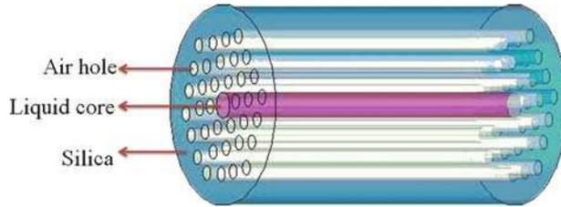
**Figure 8.** Schematic diagram of liquid-filled PCF.
