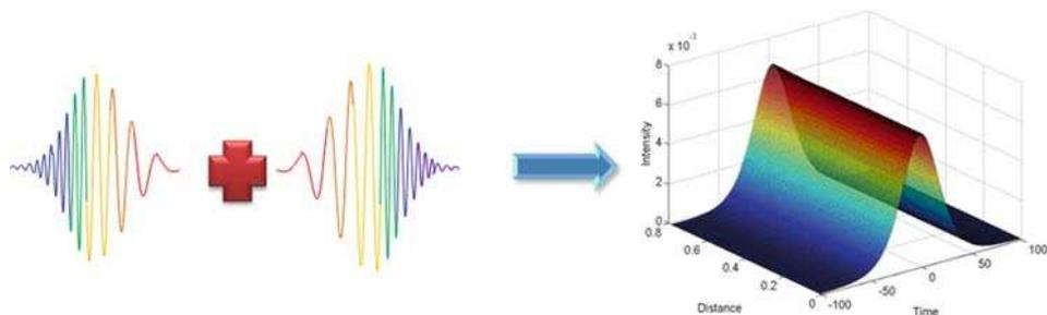
**Figure 4.** Formation of soliton by balancing the chirp induced by SPM and anomalous GVD.
