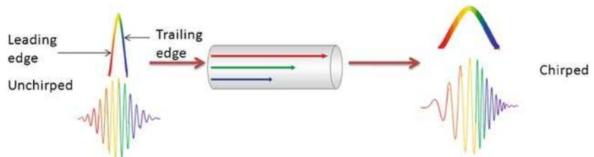
**Figure 1.** Different frequencies travel at different group velocities in fibre causing pulses to be chirped.
