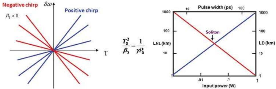
**Figure 3.** A condition can be obtained in which there is a perfect compensation of the effects. The GVD dispersion and nonlinear induced chirp have opposite signs (courtesy of google image).
