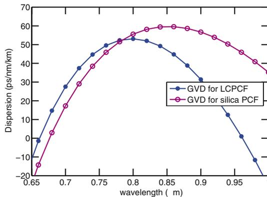
**Figure 9.** The variation of GVD for different wavelengths for both SPCF and LCPCF.
