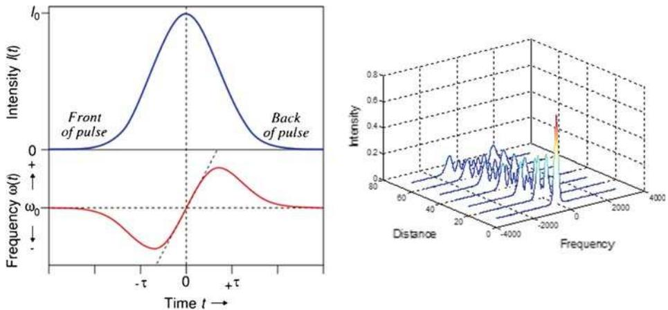
**Figure 2.** SPM acts as a positive chirp, which increases with increasing channel power level and system length (courtesy of google image).
