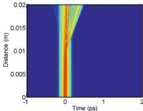
**Figure 7.** The pulse propagation through silica core PCF. The fibre parameters are  $\beta_2 = -0.0148883 \text{ ps}^2/\text{m}$ ,  $\beta_3 = 0.000032771 \text{ ps}^3/\text{m}$  and  $\beta_4 = 1.19 \times 10^{-7} \text{ ps}^4/\text{m}$ . The nonlinearity value  $\gamma = 0.04869 \text{ W}^{-1} \text{ m}^{-1}$ . The propagation length  $L = 2 \text{ cm}$ .
