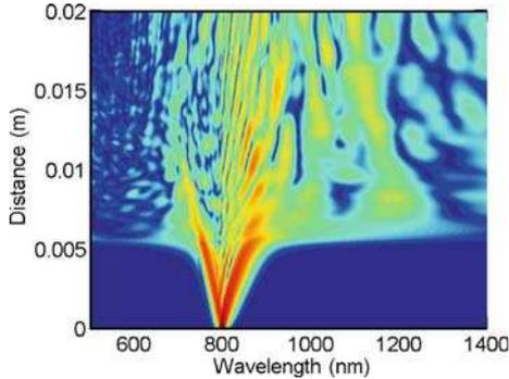
**Figure 10.** The SCG for 20 fs input pulse width in LCPCF at 800 nm. The fibre parameters are  $\beta_2 = -0.018 \text{ ps}^2/\text{m}$ ,  $\beta_3 = 0.000004850570 \text{ ps}^3/\text{m}$  and  $\beta_4 = 7.059 \times 10^{-7} \text{ ps}^4/\text{m}$ . The nonlinearity value  $\gamma = 14.56 \text{ W}^{-1} \text{ m}^{-1}$ . The propagation length  $L = 2 \text{ cm}$ .
