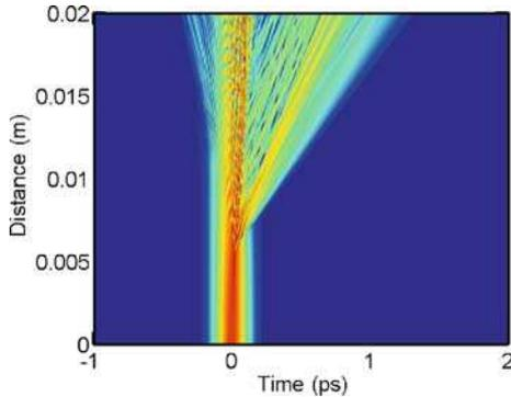
**Figure 11.** The pulse propagation through LCPCF. The fibre parameters are  $\beta_2 = -0.018 \text{ ps}^2/\text{m}$ ,  $\beta_3 = 0.000004850570 \text{ ps}^3/\text{m}$  and  $\beta_4 = 7.059 \times 10^{-7} \text{ ps}^4/\text{m}$ . The nonlinearity value  $\gamma = 14.56 \text{ W}^{-1} \text{ m}^{-1}$ . The propagation length  $L = 2 \text{ cm}$ .
