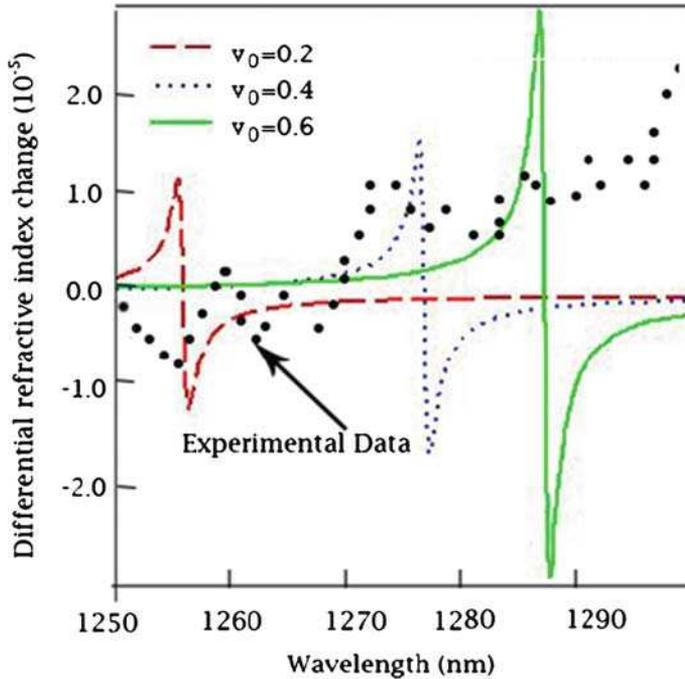
**Figure 7.** Differential refractive index changes ( $\Delta n$ ) as a function of photon wavelength for three different  $\nu_0$  with  $\alpha = 0.01$ ,  $m = 5 \text{ fm}^{-1}$ , and  $r_0 = 2$ . In this figure, we have compared our results with the experimental data (filled circles) of [52].
