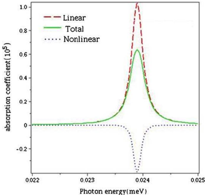
**Figure 4.** The linear, third-order nonlinear, and total absorption coefficient as a function of photon energy for  $\alpha = 0.01$ ,  $m = 5 \text{ fm}^{-1}$ ,  $r_0 = 2$ , and  $v_0 = 0.2$ .
