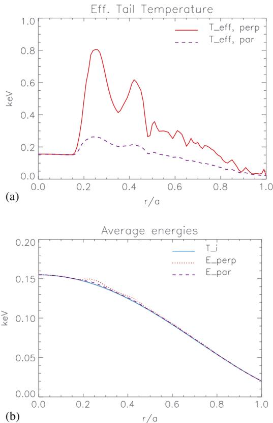
**Figure 4.** (a) Effective perpendicular temperature (solid line,  $T_{\text{eff, perp}}$ ) and parallel temperature (dashed line,  $T_{\text{eff, par}}$ ) profiles, (b) average perpendicular energy (dotted line,  $E_{\text{perp}}$ ) and parallel energy (dashed line,  $E_{\text{par}}$ ) profiles of hydrogen ions due to the total coupled power of 0.044 MW. The initial ion temperature profile (solid line,  $T_i$ ) is also shown.
