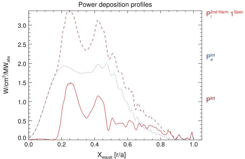
**Figure 1.** Radial power deposition profiles of shot #20685 evaluated by TORIC. The curve  $P_i^{2ndHarm | Spec}$  (solid line) shows the power deposition profile of ions due to second-harmonic heating whereas the curve  $P_e^{tot}$  (dotted line) shows the total power deposition profile of electrons. The curve  $P^{tot}$  (dashed line) represents the profile of total power absorbed. The total power is normalized to 1 MW.
