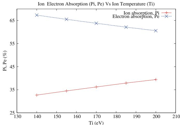
**Figure 5.** Ion and electron power absorption (in %),  $P_i$  and  $P_e$  respectively, with ion temperature ( $T_i$ ).
