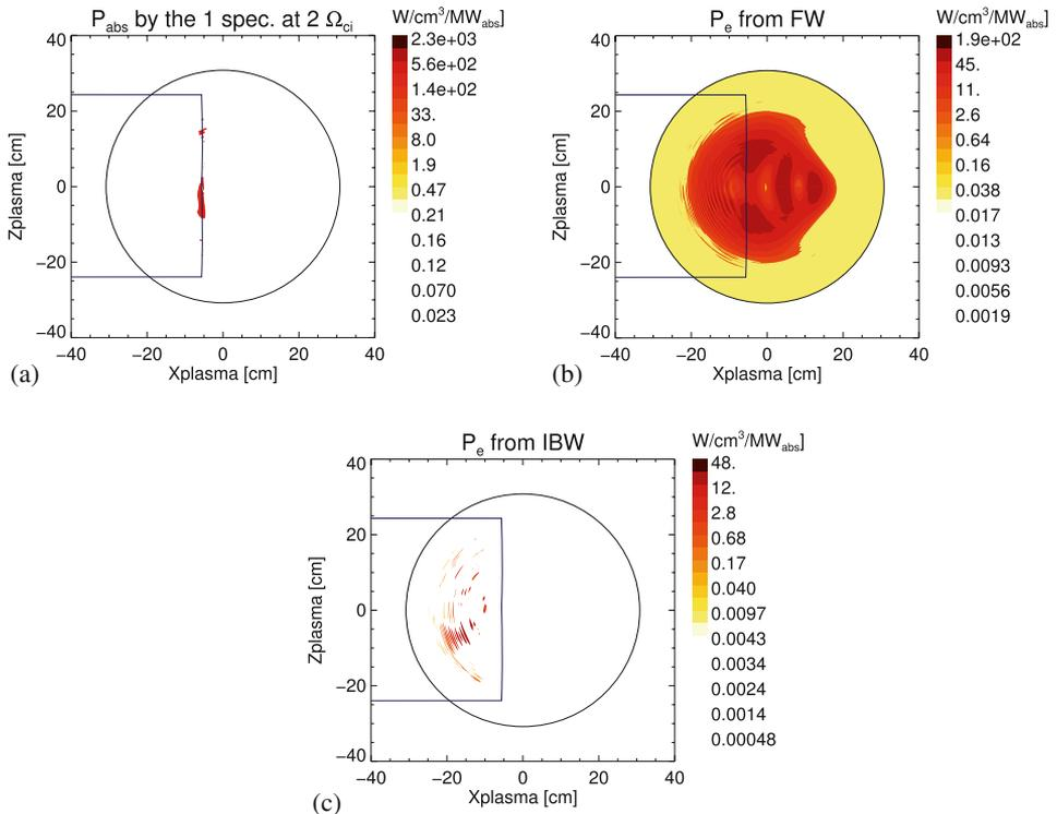
**Figure 2.** Power absorbed by (a) ions at the second-harmonic from FW, (b) electrons from FW, (c) electrons from IBW in the poloidal cross-section as evaluated by TORIC. The vertical line indicates the second-harmonic resonance layer for hydrogen ions.
