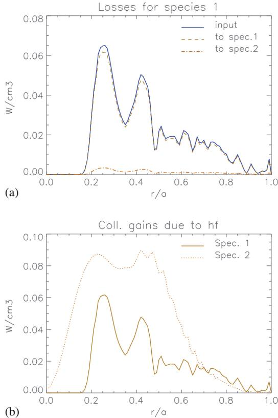
**Figure 6.** (a) Collisional power losses of rf-heated hydrogen ions (solid line, 'input') to the background ion (dashed line, 'to spec. 1') and electrons (dot-dashed line, 'to spec. 2'), (b) the power profiles of ions (solid line, 'spec. 1') and electrons (dotted line, 'spec. 2') due to collisional gain.
