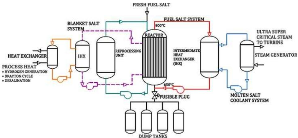
**Figure 7.** Preliminary lay-out of the proposed loop-type Indian MSBR.
