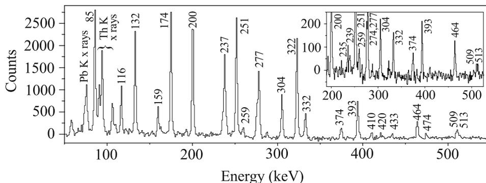
**Figure 5.** Gamma-ray transitions from positive- and negative-parity states in the yrast octupole structure of  $^{221}\text{Th}$ .
