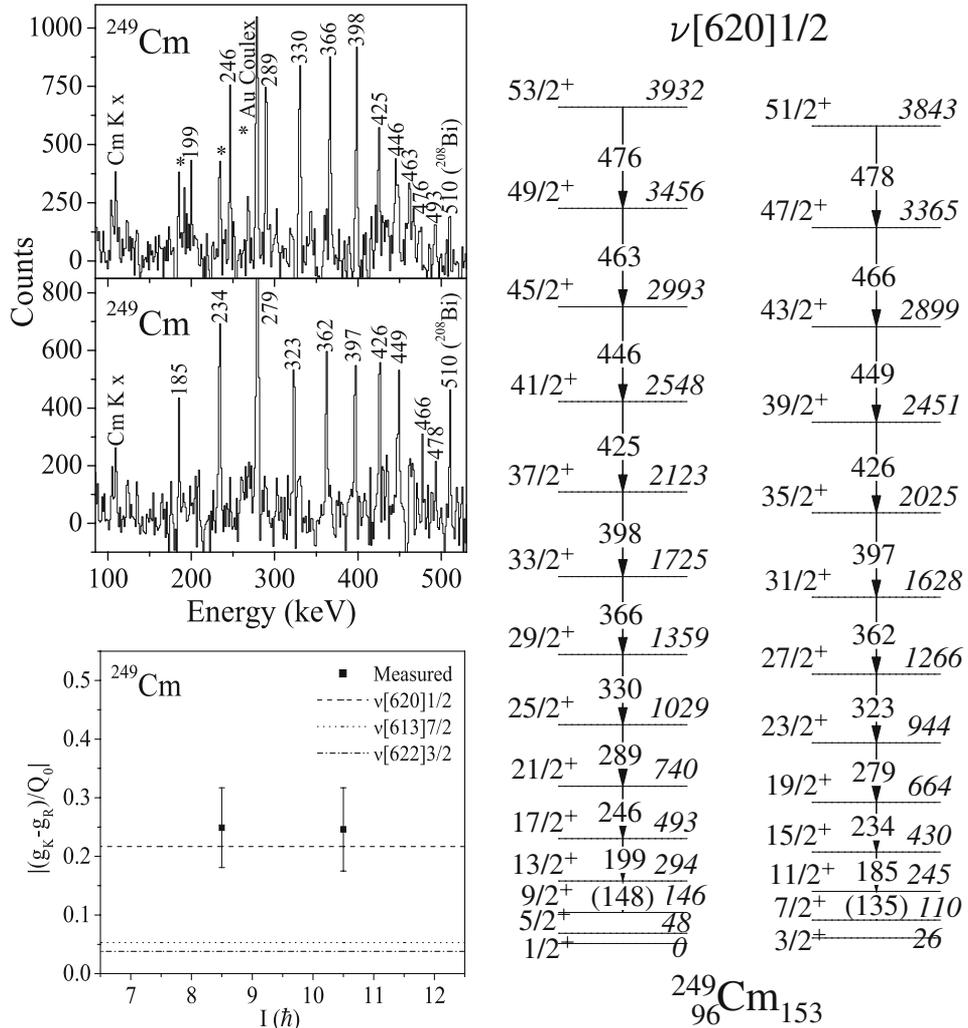
**Figure 2.** Gamma-ray coincidence spectra and partial decay scheme for  ${}^{249}\text{Cm}$ . The observed rotational band is built on the  $\nu[620]1/2$  ground state. Though  $\Delta I = 1$  transitions were not observed,  $(g_K - g_R)/Q_0$  values for the two states could be deduced from the observed coincidences between signature partners.
