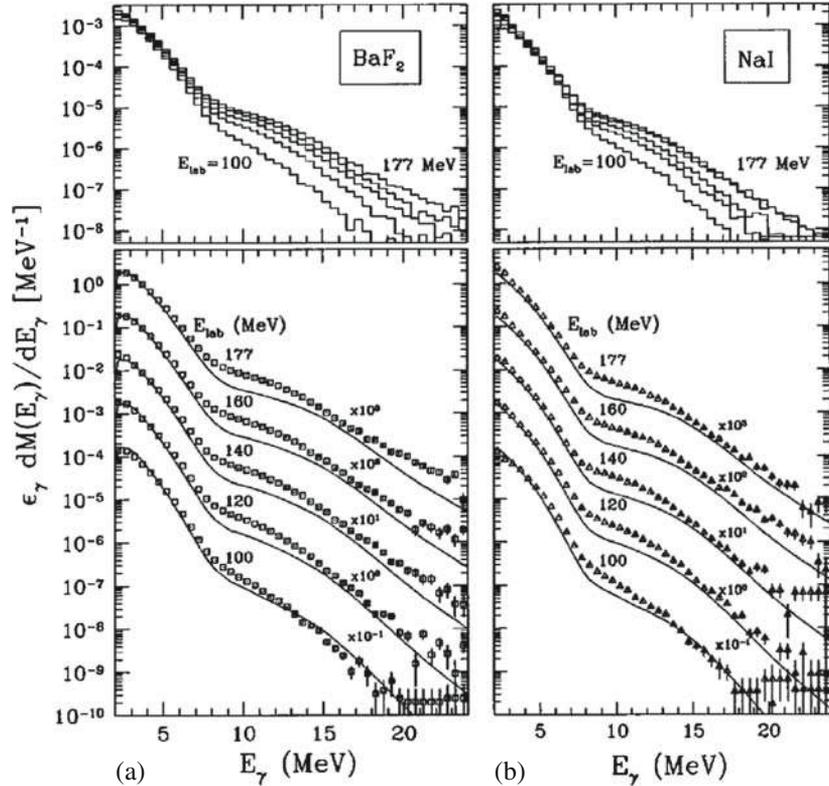
**Figure 1.** Absolute  $\gamma$ -ray/fission multiplicities for the  $^{16}\text{O} + ^{208}\text{Pb}$  reaction measured in  $\text{BaF}_2$  array (a) and large volume  $\text{NaI(Tl)}$  detector (b). The solid lines are CASCADE calculations without viscosity.
