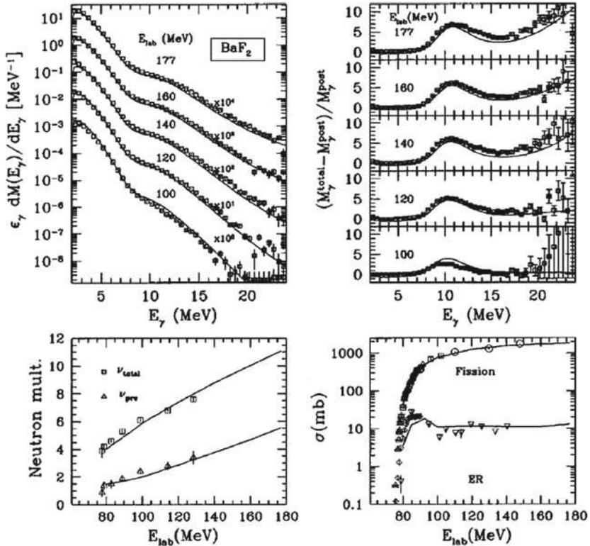
**Figure 2.**  $\gamma$ , neutron multiplicities and ER cross-sections for the  $^{16}\text{O} + ^{208}\text{Pb}$  reaction compared with the calculations including temperature-dependent ( $T^2$ ) viscosity parameter  $\gamma$  and a strong temperature-dependent nuclear level density.
