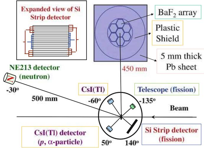
Figure 1. Schematic representation of the experimental set-up (see text).
