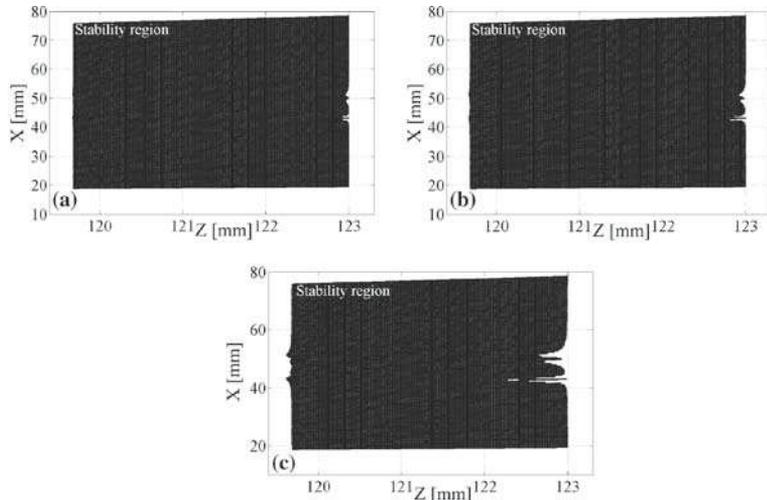
**Figure 3.** The black colour indicates the common stability region between the sagittal and tangential planes vs. the central resonator length ( $Z$ ) and the rod position ( $X$ ) for (a)  $P = 0.5P_{cr}$ , (b)  $P = P_{cr}$  and (c)  $P = 4P_{cr}$ .
