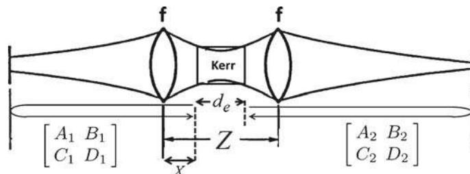
**Figure 2.** Linear resonator configuration of KLM laser. The matrices represent the propagation from the face of the Kerr rod to the corresponding end mirror and back to the face of the rod.
