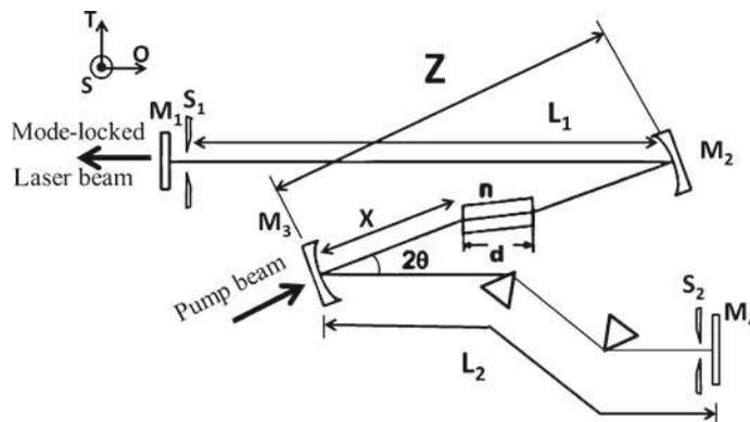
**Figure 1.** Resonator configuration for KLM laser: tilted mirrors  $M_2$  and  $M_3$  are focussing; output mirror  $M_1$  and back mirror  $M_4$  are flat;  $S_1$  and  $S_2$  are the slits;  $L_1$  and  $L_2$  are the arms. The Kerr medium is placed between the mirrors  $M_2$  and  $M_3$  in the central resonator.
