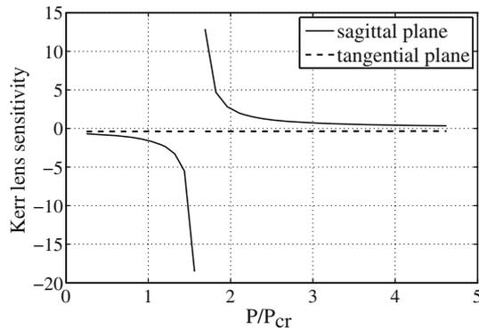
**Figure 4.** Kerr lens sensitivity vs. resonator input power in optimum operation.
