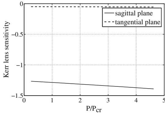
**Figure 5.** Kerr lens sensitivity vs. resonator input power for normal operation.
