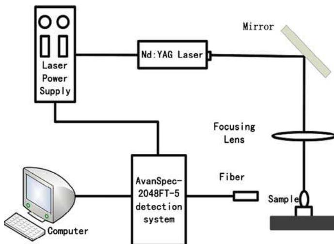
Figure 1. LIBS set-up for experiments.
