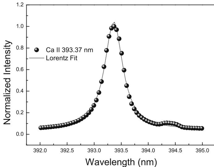
**Figure 6.** Stark-broadened profile of Ca II 393.37 nm in laser-induced egg shell plasma.
