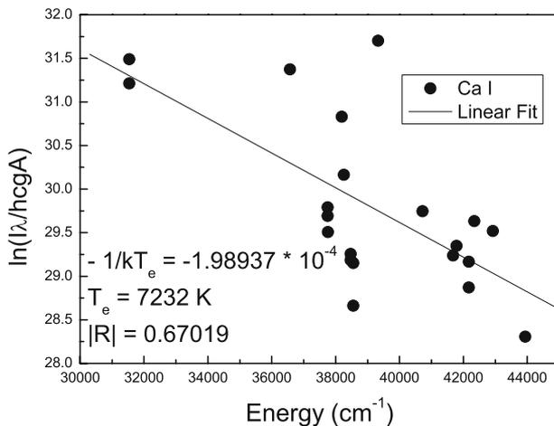
**Figure 3.** Boltzmann plot with 21 Ca I emission lines in laser-induced egg shell plasma. The fitting correlation coefficient  $R = 0.67019$ .
