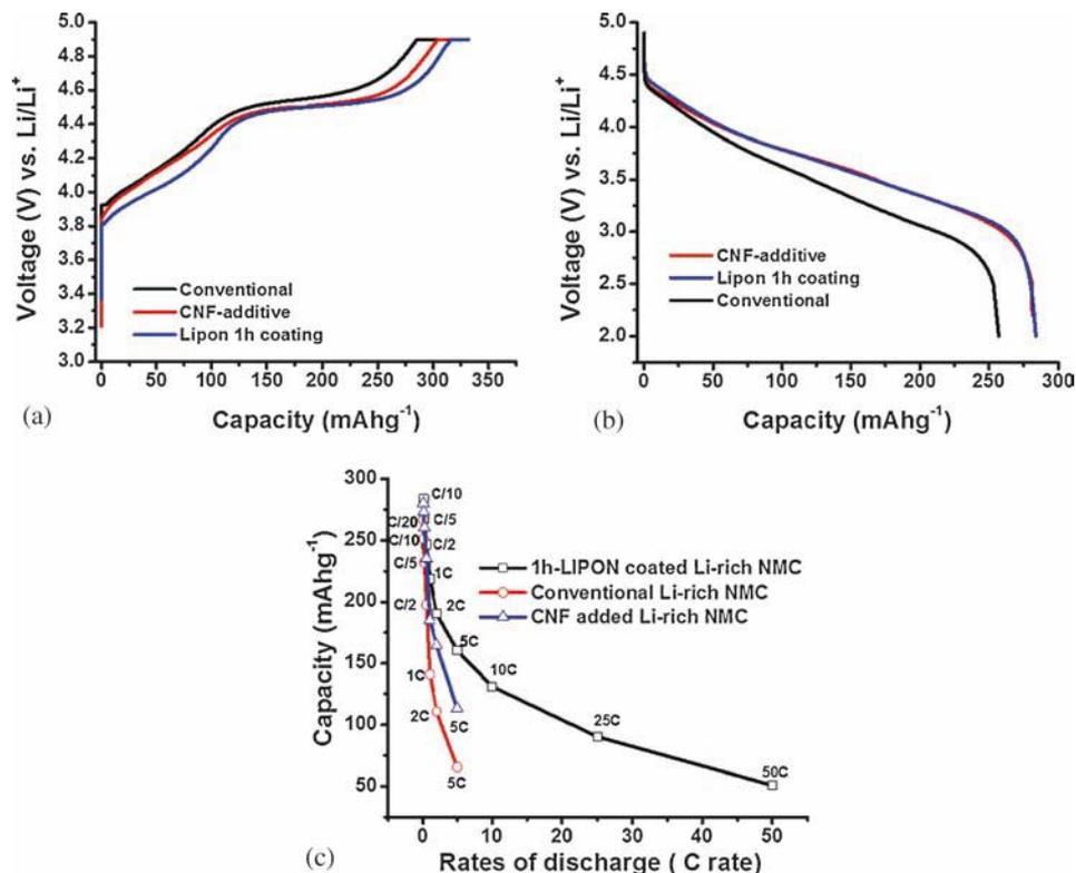
**Figure 5.** (a) Charge and (b) discharge voltage profiles of LMR–NMC composite electrodes measured galvanostatically at  $C/10$  rate during first cycles at 4.9 V cut-off for conventional, CNF-added and lipon-coated electrodes at  $25^\circ\text{C}$ . (c) Comparison of rate capabilities (discharge capacity vs. rates) for conventional and CNF added and lipon coated on to LMR–NMC particle composite electrodes measured galvanostatically at various rates (as indicated) at  $25^\circ\text{C}$ .
