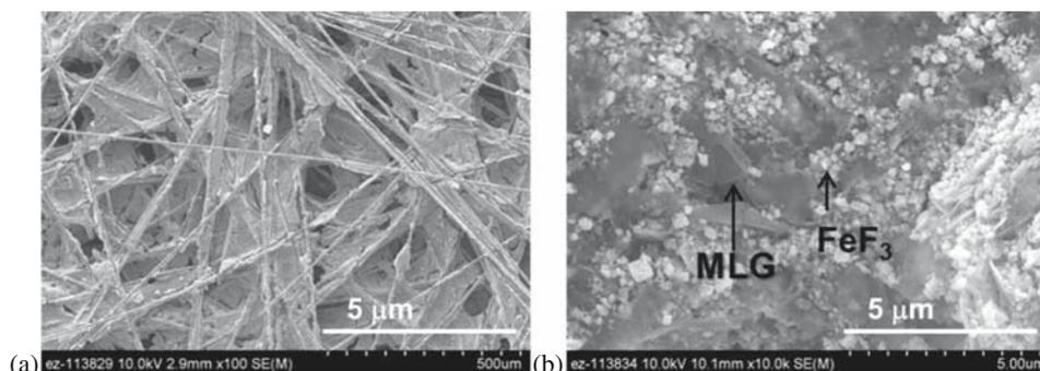
**Figure 7.** SEM and STEM images showing typical shapes and sizes of  $\text{FeF}_2$  and  $\text{FeF}_3$  particles and electrodes. (a) Pristine  $\text{FeF}_3/\text{FeF}_2$ –MLG carbon fibre electrode, (b)  $\text{FeF}_3$  and MLG after electrode fabrication at  $450^\circ\text{C}$ .
