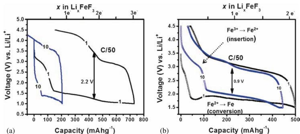
**Figure 8.** Voltage vs. capacity profiles of Li/FeF<sub>3</sub> cell on (a) FeF<sub>3</sub> slurry coated on Al foil, (b) FeF<sub>3</sub> supported on carbon fibre electrodes cycled between 1 V/1.5 V and 4.5 V (C/50 rate) at 25°C.
