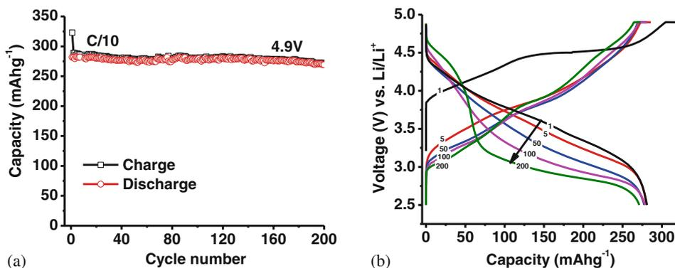
**Figure 6.** (a) Charge–discharge cycling of LMR–NMC composite electrodes measured galvanostatically at  $C/10$  rate and 4.9 V cut-off for CNF-added electrodes at  $25^{\circ}\text{C}$ . (b) Voltage profiles of CNF-added LMR–NMC composite electrodes measured galvanostatically at  $C/10$  rate during 200 cycles (cycle numbers are indicated in the voltage profiles) at  $25^{\circ}\text{C}$ . The cycling protocol was the same as above.
