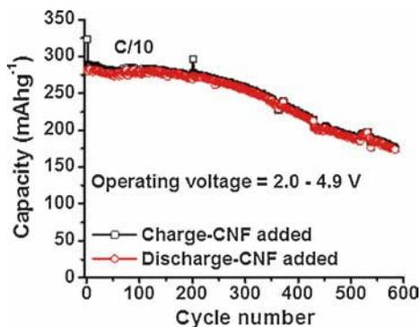
**Figure 4.** Charge–discharge cycling data at various potentials (as indicated) of LMR–NMC composite electrodes at  $C/10$  rate, in EC-DMC 1:2/LiPF<sub>6</sub> 1.2 M solutions (coin-type cell,  $T = 25^{\circ}\text{C}$ ). The cycling protocol was the same as described in figure 3.
