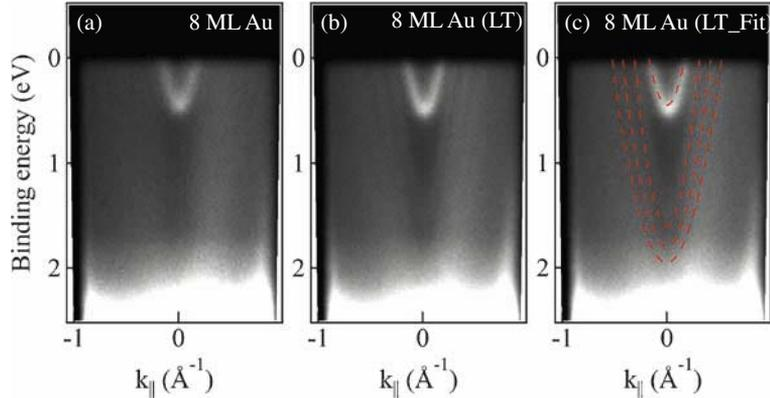
**Figure 5.** ARPES spectra of (a) 8 ML of Au grown on graphite surface at RT, (b) 8 ML of Au film grown on graphite at LT and annealed to RT and (c) same as that of (b) with fitted lines for SS and QW features. See text for details.
