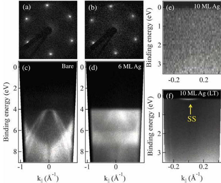
**Figure 2.** LEED pattern at  $E_p = 140$  eV of (a) cleaved graphite(0001) surface, (b) 6 ML of Ag grown on graphite at RT. ARPES spectra of (c) *in-situ* cleaved graphite(0001) surface along  $\Gamma M$  direction, (d) 6 ML of Ag film grown on graphite at RT, (e) 10 ML of Ag film grown on graphite at RT, (f) 10 ML of Ag film grown on graphite at LT and annealed to RT, with intense SS shown by yellow arrow.
