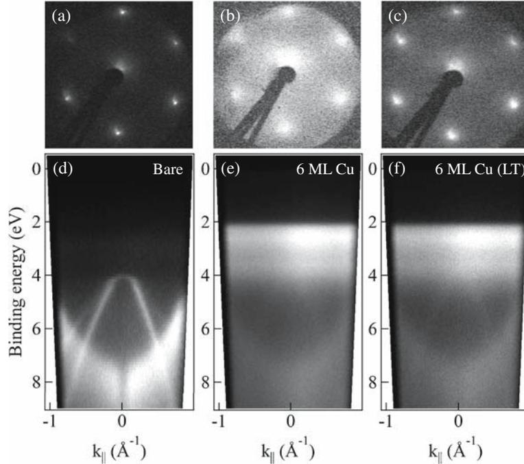
**Figure 1.** LEED pattern at primary energy 140 eV of (a) *in-situ* cleaved graphite(000 1) surface, (b) 6 ML of Cu grown on graphite at RT, (c) 6 ML of Cu grown on graphite surface at LT and annealed to RT. ARPES spectra of (d) *in-situ* cleaved graphite, (e) 6 ML of Cu film grown on graphite at RT, (f) 6 ML of Cu film grown on graphite at LT and annealed to RT.
