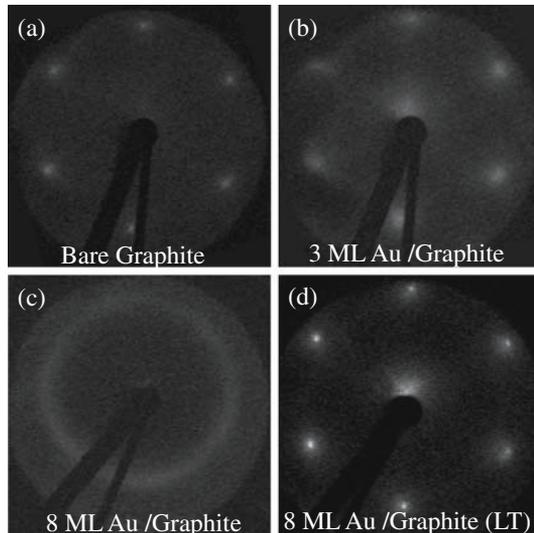
**Figure 3.** LEED pattern at  $E_p = 140$  eV of (a) cleaved graphite(0001) surface, (b) 3 ML of Au, (c) 8 ML of Au, grown on graphite surface at RT and (d) 8 ML of Au, grown on graphite surface at LT and annealed to RT.
