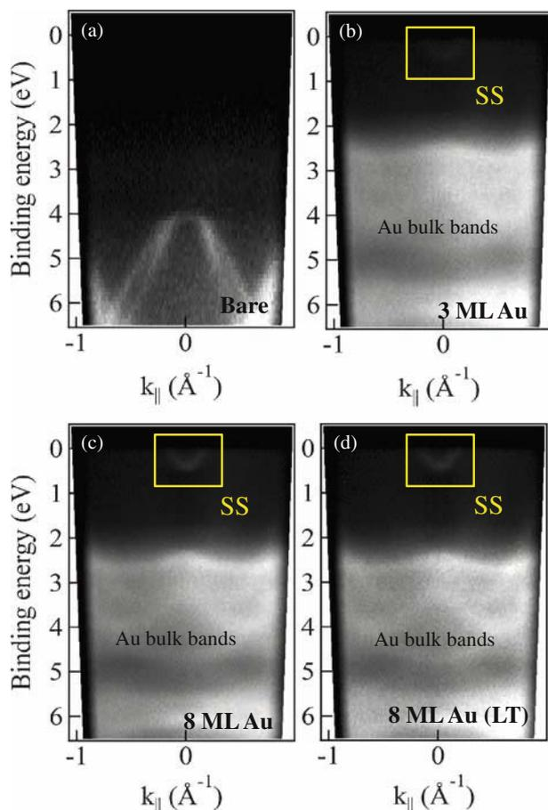
**Figure 4.** ARPES spectra of (a) *in-situ* cleaved graphite(0001) surface along  $\Gamma M$  direction, (b) 3 ML of Au, (c) 8 ML of Au film, grown on graphite at RT and (d) 8 ML of Au grown on graphite at LT annealed to RT. Yellow boxes indicate the Au SS.
