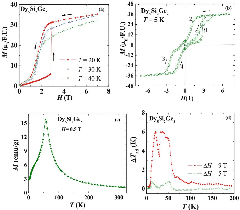
**Figure 3.** (a,b) Magnetization vs. field for  $Dy_5Si_2Ge_2$  compound at selected temperatures (the numbers and arrows in the figure indicate the field cycle path), (c) magnetization vs. temperature for  $Dy_5Si_2Ge_2$  in 0.5 T field and (d) change in adiabatic temperature vs. temperature for  $Dy_5Si_2Ge_2$  (ref. [39]).
