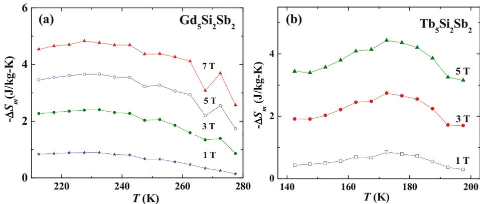
**Figure 1.** Change in isothermal magnetic entropy vs. temperature for (a) Gd<sub>5</sub>Si<sub>2</sub>Sb<sub>2</sub> and (b) Tb<sub>5</sub>Si<sub>2</sub>Sb<sub>2</sub> compounds near  $T_C$  for various magnetic field changes (from refs [32,33]).
