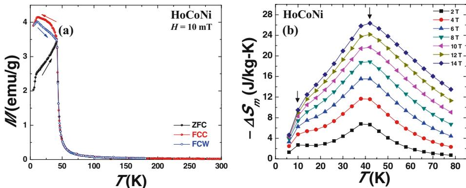
**Figure 2.** (a) Magnetization vs. temperature of  $\text{HoCoNi}$  compound in 10 mT field measured in zero-field-cooled (ZFC) and field-cooled cooling (FCC) and warming (FCW) cycles and (b) isothermal magnetic entropy change vs. temperature of  $\text{HoCoNi}$  for various magnetic field changes (ref. [34]).
