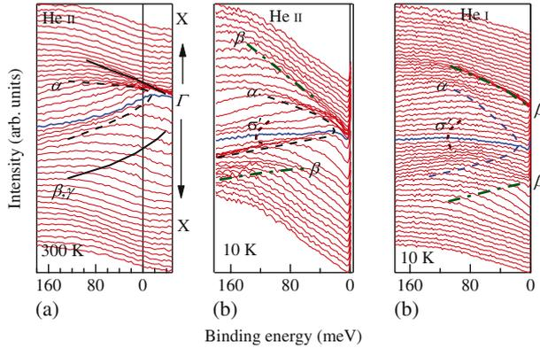
**Figure 5.** Energy distribution curves (EDCs) in the He II spectra at (a) 300 K and (b) 10 K. (c) The EDCs in the He I spectra at 10 K.
