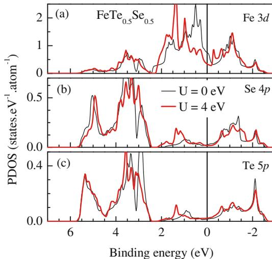
**Figure 3.** Calculated (a) Fe  $3d$ , (b) Se  $4p$  and (c) Te  $5p$  partial density of states for uncorrelated (thin line for  $U = 0$  eV) and correlated systems (thick line for  $U = 4.0$  eV).
