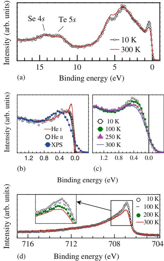
**Figure 2.** (a) XP valence band spectrum of  $\text{FeTe}_{0.6}\text{Se}_{0.4}$  at 300 K (line) and 10 K (symbols). (b) Near-Fermi level spectra at 10 K obtained using He I, He II and Al  $K\alpha$  lines at 10 K. (c) Temperature evolution of the near-Fermi level XP feature. (d) Fe  $2p$  core level spectra. Inset shows expanded view of the well-screened feature.
