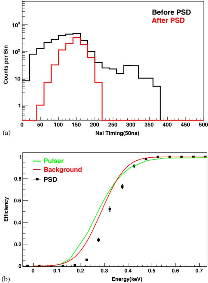
**Figure 4.** (a) Relative timing between AC-NaI(Tl) and PCGe systems, before and after PSD selection. The ‘50–200 ns’ is the coincidence window where the signals at PCGe are mainly due to physics events correlated with the AC detector. (b) PSD selection efficiencies were derived from the survival probabilities of AC-tagged events. The trigger efficiencies of the 500-g PCGe detector, as derived from the test pulser and *in-situ* background events.
