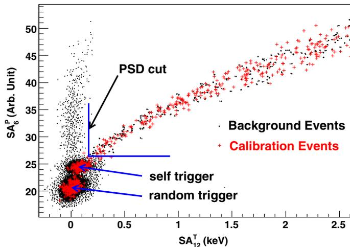
**Figure 3.** Scattered plots of the  $SA_6^P$  (shaping time is 6  $\mu s$  with partial integration) vs.  $SA_{12}^T$  (shaping time is 12  $\mu s$  with partial integration) signals, for both calibration and physics events. The PSD selection is shown.
