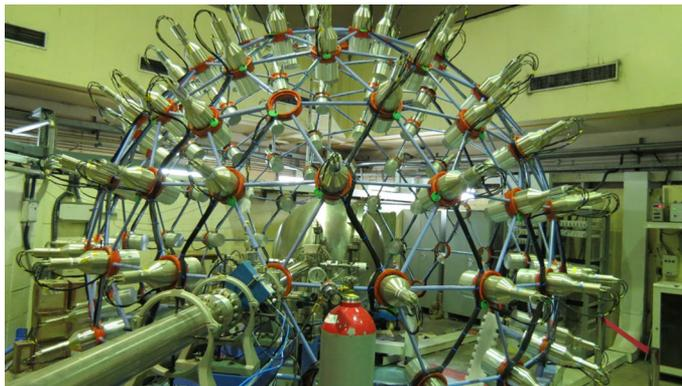
**Figure 1.** The detector array installed in the beam line.
