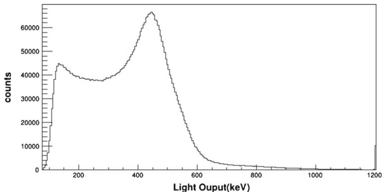
**Figure 3.** Light output from a  $5'' \times 5''$  liquid scintillator detector irradiated by 662 keV  $\gamma$ -rays from  $^{137}\text{Cs}$  source.
