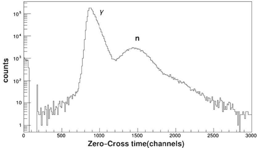
Figure 4. Neutron  $\gamma$  separation by zero-cross time distribution.
