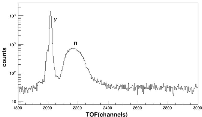
**Figure 6.** TOF spectrum showing separation of neutrons and  $\gamma$ -rays from  $^{252}\text{Cf}$  source.
