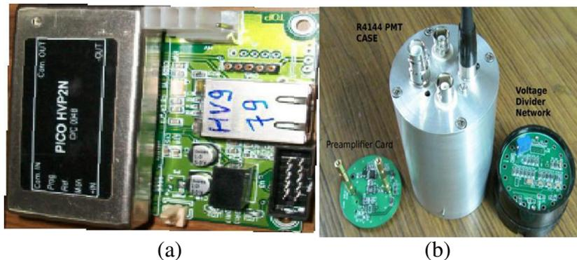
**Figure 2.** (a) A single-channel high voltage power supply and (b) PMT base with the voltage divider and the preamplifier.
