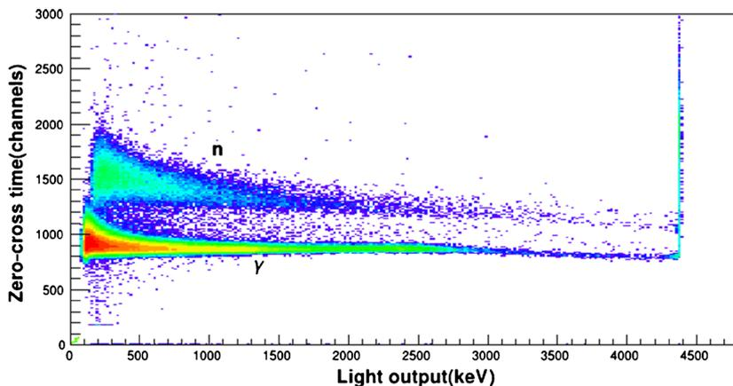
Figure 5. PSD (zero-cross time) plotted against light output.
