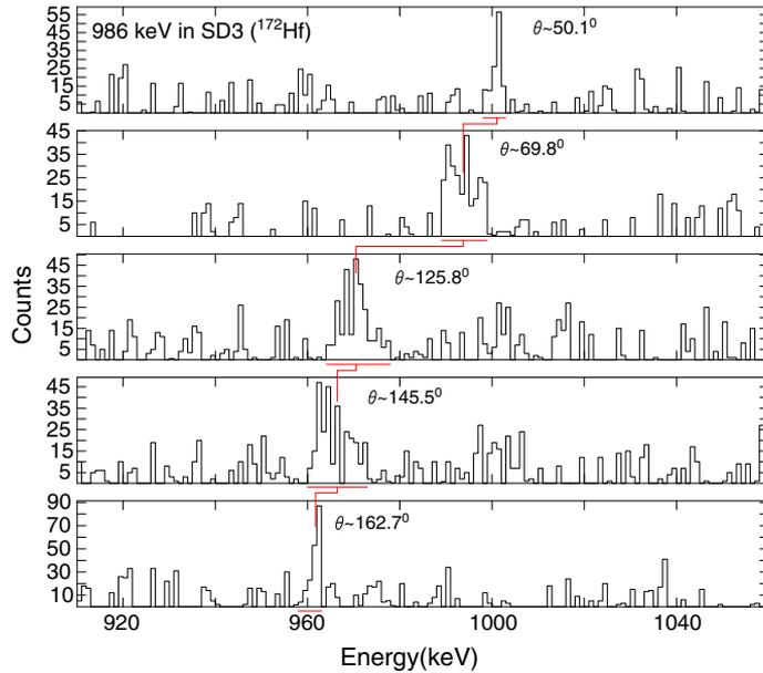
**Figure 3.** Representative, summed coincidence  $\gamma$ -ray spectra profile for the 986-keV transition in SD3 at different angles. An average detector angle is shown where two close lying rings of Gammasphere were summed for better enhancement of the peak shape.
