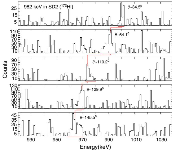
**Figure 2.** Representative, summed coincidence  $\gamma$ -ray spectra profile for the 982-keV transition in SD2 at different angles. An average detector angle is shown where two close lying rings of Gammasphere were summed for better enhancement of the peak shape.
