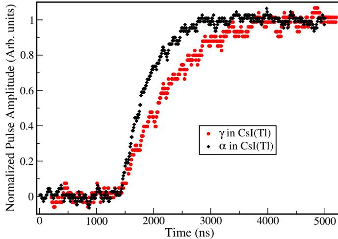
**Figure 7.** Preamplifier pulses from the CsI(Tl) detector stored in the DDAQ originating from the interaction of the  $\alpha$ -particles (black) and  $\gamma$ -rays (red) in the detector.
