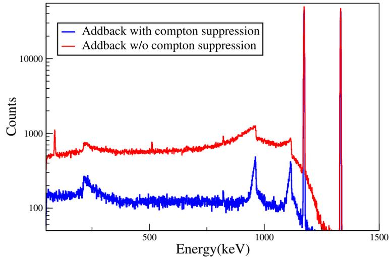
**Figure 2.** Simulated add-back spectra of  $^{60}\text{Co}$  in clover with and without Compton suppression.
