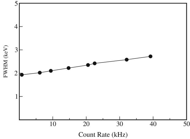
**Figure 3.** Variation of FWHM of 1173 keV transition emitted in the decay of  $^{60}\text{Co}$  at different count rates using the present DDAQ. A two-source method has been used to study the effect of high count rate on the energy resolution of  $\gamma$ -rays.
