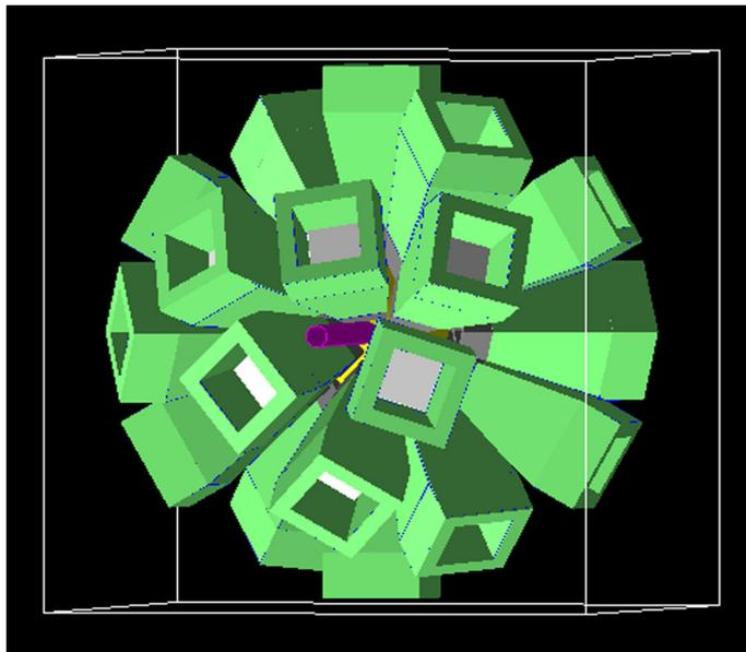
**Figure 1.** Geometry of the 24 Compton-suppressed clovers of the INGA at TIFR–BARC Pelletron Linac Facility used in the GEANT4 simulation.
