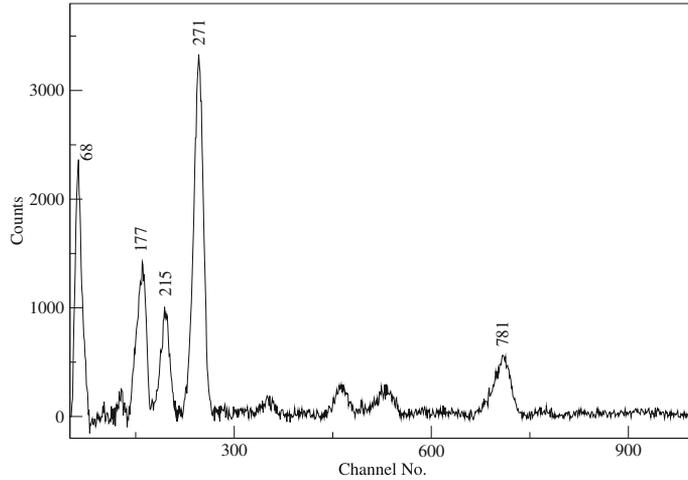
**Figure 5.** LaBr<sub>3</sub>(Ce) spectrum obtained with gate on 1944 keV transition of <sup>89</sup>Zr is depicted. The strong lines of <sup>89</sup>Zr are marked in the spectrum.
