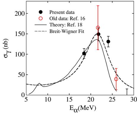
**Figure 4.** Extracted  $\gamma$ -transition cross-sections plotted against the effective  $\alpha$ -particle energy (see text). The last point indicates the upper bound of the cross-section. The continuous line shows the result of the cluster model with Buck potential. The dashed line shows the Briet–Wigner fit to the data.
