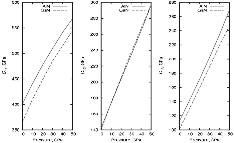
**Figure 4.** Elastic constants  $C_{11}$ ,  $C_{12}$  and  $C_{13}$  are shown at different pressures for wz-AlN and wz-GaN. For wz-AlN,  $C_{11}$  and  $C_{13}$  are higher when compared to wz-GaN and similar for  $C_{12}$ .
