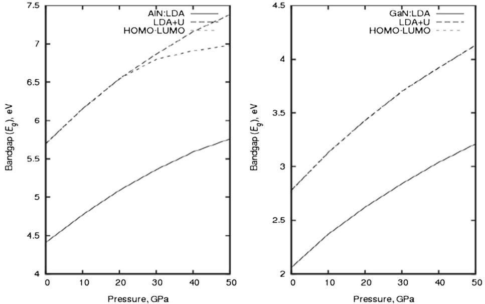
**Figure 8.** Band-gap variation vs. pressure for wz-AlN and wz-GaN. AlN: LDA band gap with LDA pseudopotential, LDA+ $U$  band gap with LDA+ $U$  correction and HOMO–LUMO effect has been observed after 20 GPa in wz-AlN but HOMO-LUMO splitting in wz-GaN has not been observed till 50 GPa.
