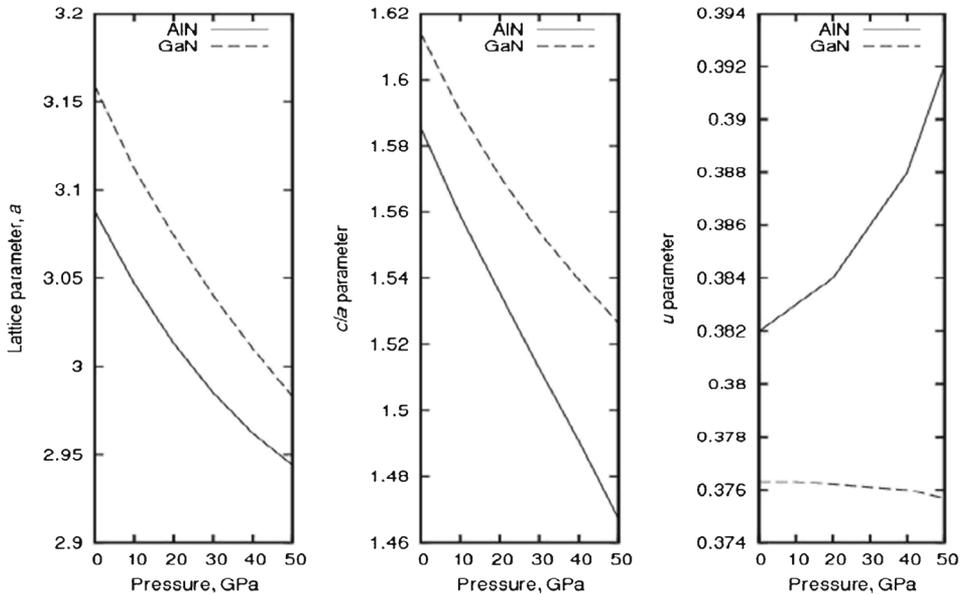
**Figure 3.** Variations of lattice parameter ( $a$ ),  $c/a$  and  $u$  at different pressures are shown for wz-AlN and wz-GaN. All these parameters decrease except  $u$  which increases for wz-AlN and slightly decrease for wz-GaN as pressure increases.
