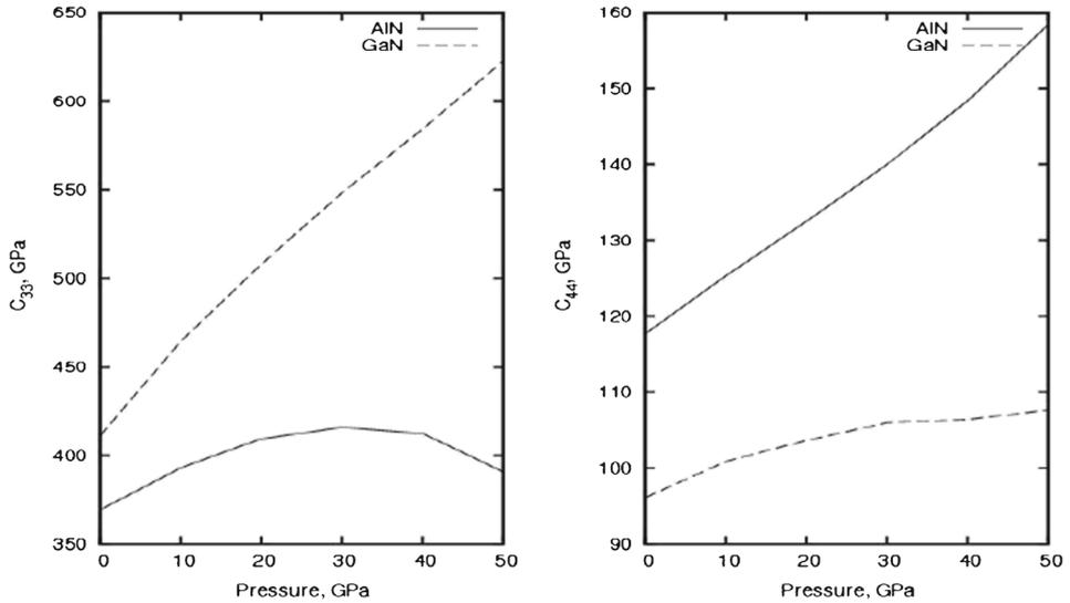
**Figure 5.** Elastic constants  $C_{33}$  and  $C_{44}$  are shown at different pressures for wz-AlN and wz-GaN.  $C_{33}$  increases linearly for wz-GaN but decreases for wz-AlN as pressure increases and  $C_{44}$  for wz-AlN is higher when compared to wz-GaN.
