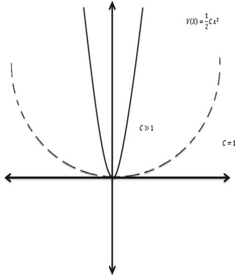
**Figure 1.** Quantum dot confinement potential. For  $C \gg 1$  the confinement potential is very thin.
