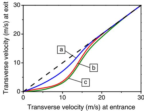
**Figure 3.** Transverse velocity of metastable Kr atoms at the exit of the collimator as a function of the transverse velocity at the entrance of collimator for (Curve a) laser beam width  $w \sim 7$  mm, (Curve b) laser beam width  $w \sim 25$  mm and (Curve c) continuous interaction case ( $\Delta_L/2\pi = +10$  MHz,  $\beta_0 = 70$  mrad,  $\alpha = 5$  mrad,  $d = 120$  mm,  $v_L = 300$  m/s,  $\lambda = 811.5$  nm). The straight dashed line represents the absence of transverse cooling.
