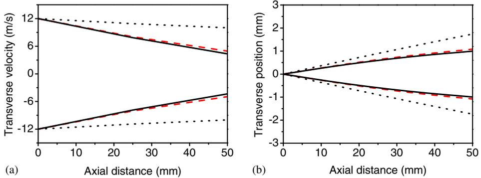
**Figure 2.** (a) Transverse velocity vs. axial distance and (b) transverse position vs. axial distance, for laser beam width of  $w = 25$  mm (dashed curve) and  $w = 7$  mm (dotted curve) ( $\Delta_L/2\pi = +10$  MHz,  $\beta_0 = 70$  mrad,  $\alpha = 5$  mrad,  $d = 120$  mm,  $v_L = 300$  m/s and  $\lambda = 811.5$  nm). The solid line represents the continuous interaction case.
