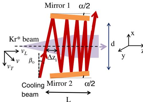
**Figure 1.** The zig-zag atomic beam collimator for a larger laser incidence angle showing discrete interaction of laser beam with Kr\* atomic beam. Here,  $\beta_0$  is the incident laser beam angle,  $\alpha$  is the mirror angle,  $d$  is the separation between mirrors of length  $L$  and  $\Delta z_i$  is the length of non-interacting region.
