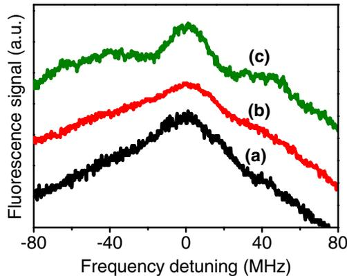
**Figure 5.** Effect of cooling laser beam width ( $w$ ) on the transverse cooling of the metastable  $^{84}\text{Kr}^*$  atomic beam. (Curve a) Transverse cooling beam is absent, (Curve b)  $w = 7$  mm and (Curve c)  $w = 25$  mm ( $\Delta_L/2\pi = +10$  MHz,  $\beta_0 = 70$  mrad,  $d = 120$  mm,  $v_L = 300$  m/s,  $\lambda = 811.5$  nm and  $\alpha = 5$  mrad).
