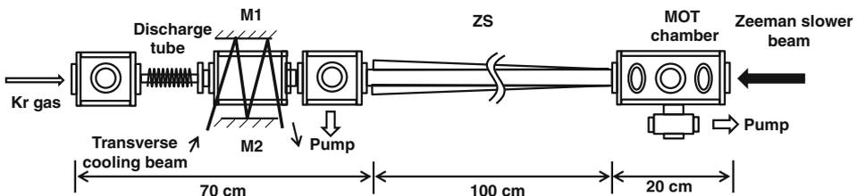
Figure 4. The schematic of the experimental set-up used for cooling  $\text{Kr}^*$  atoms.
