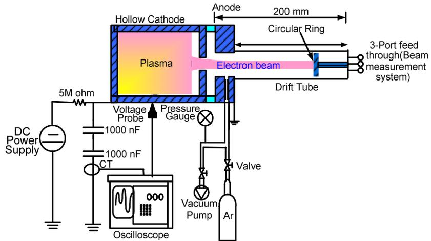
**Figure 1.** Schematic view of the experimental set-up.
