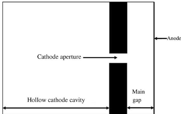
**Figure 4.** Electrode geometry of PCE-Gun as taken in the simulations.
