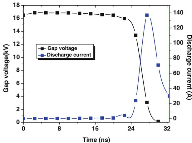
**Figure 5.** Trace of discharge current and gap voltage obtained from simulations.
