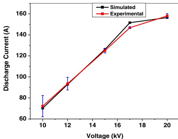
**Figure 7.** Variation of discharge current with applied voltage.
