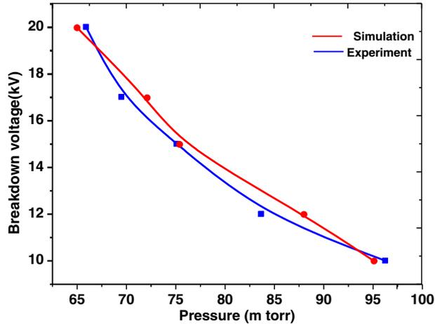
**Figure 6.** Breakdown voltage with gas pressure for argon at 59.7 mm cathode cavity depth, 3 mm gap separation and 3 mm cathode aperture.
