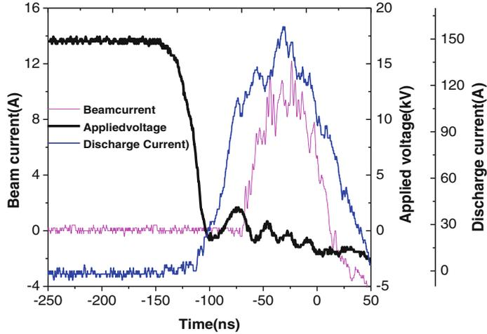
**Figure 3.** Experimentally observed profile of discharge current, beam current (measured at  $z = 107$  mm) and gap voltage.
