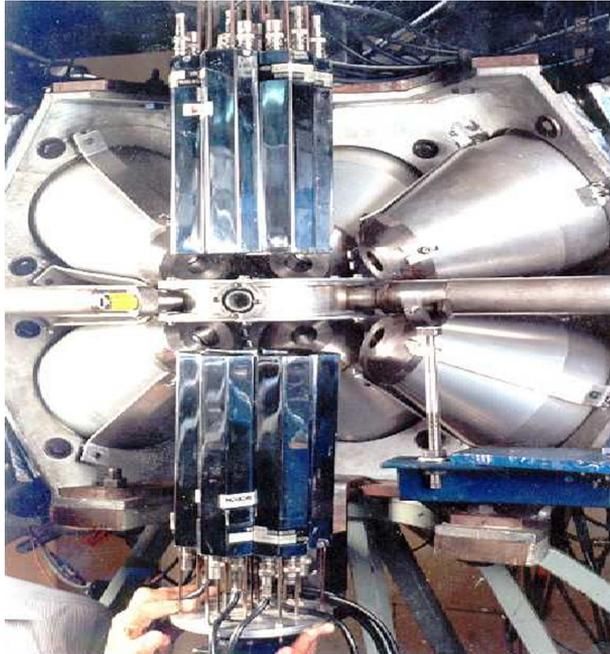
**Figure 2.** Inside view of GDA with scattering chamber and fourteen-element BGO multiplicity filter.
