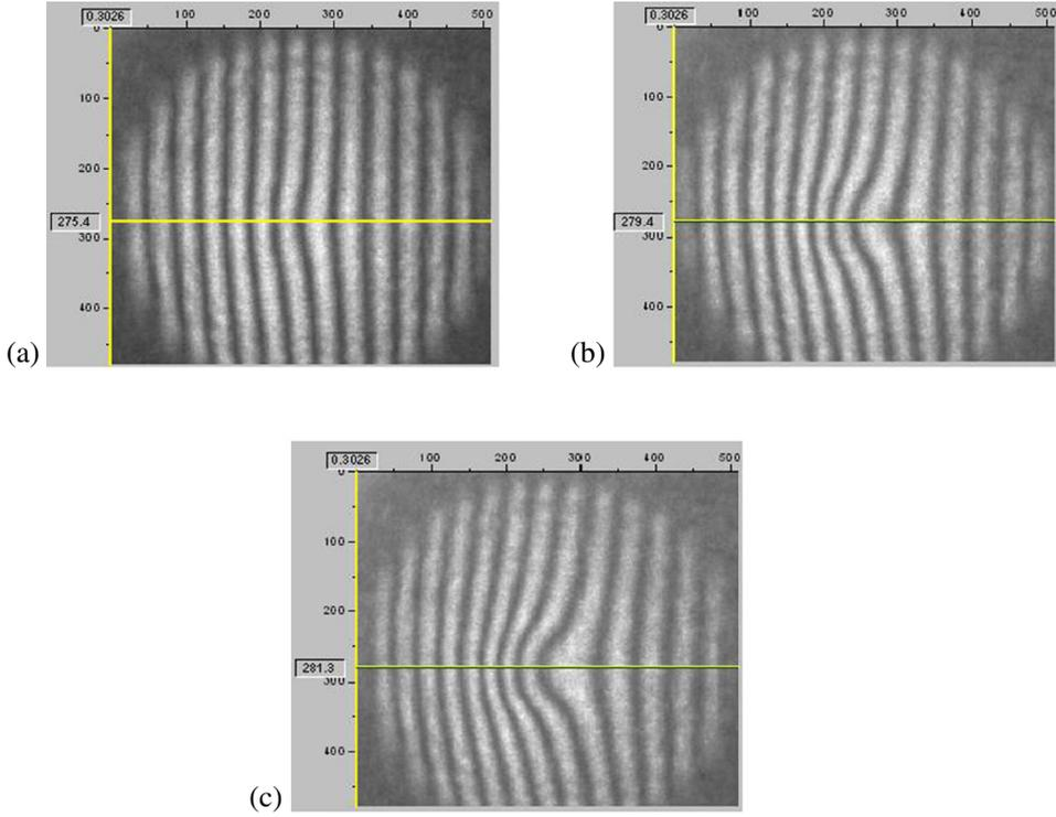
**Figure 3.** Interferograms obtained for a power density of (a) 20.9 W/cm<sup>2</sup>, (b) 56.0 W/cm<sup>2</sup> and (c) 78.4 W/cm<sup>2</sup> (initial spot size ~5 mm).
