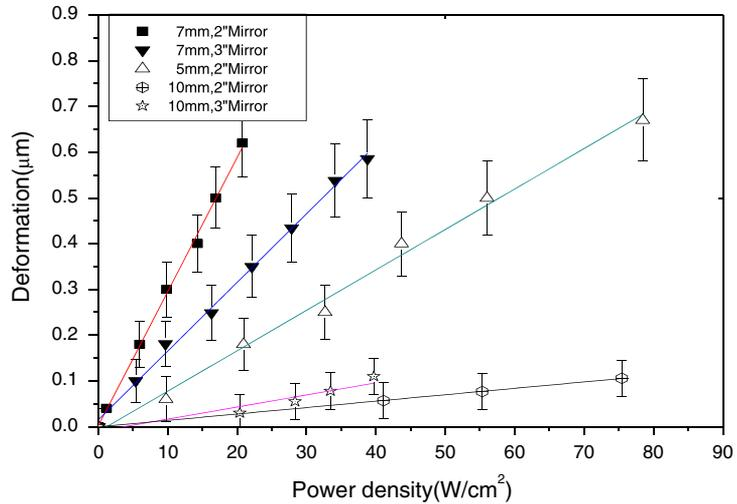
**Figure 4.** Deformation vs. average power density for mirrors with BK7 substrate. The inset data show spot size and mirror diameter.
