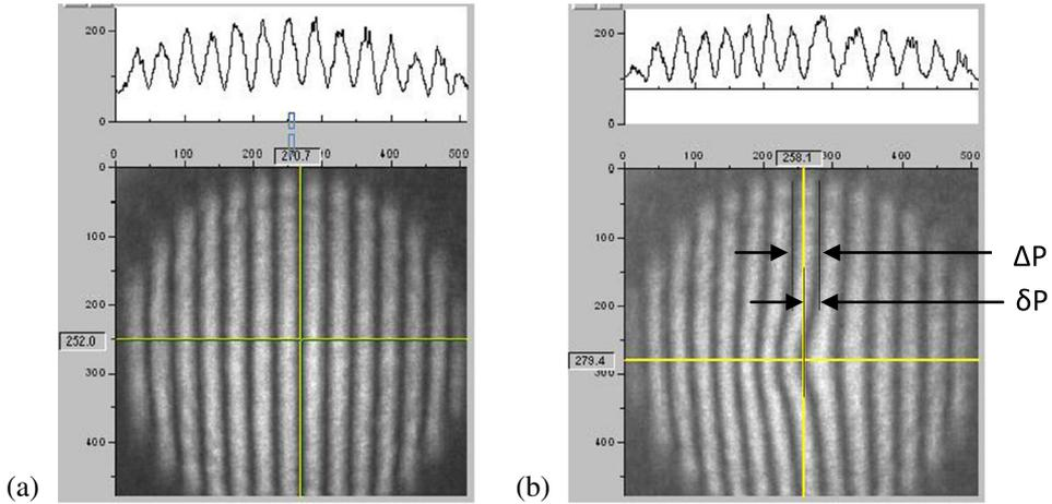
**Figure 2.** Interferogram (a) reference (without CVL), (b) with CVL (7.7 W, 5 mm spot size).
