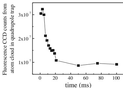
**Figure 2.** Variation in the number of atoms trapped with time in quadrupole magnetic trap for  $\sim 13$  A of current in the coils.
