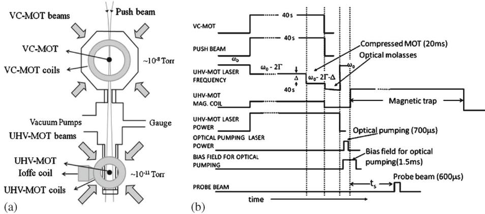
**Figure 1.** Schematic of the experimental set-up (a) and the sequence of pulses (b) used for magnetic trapping of  $^{87}\text{Rb}$  atoms.
