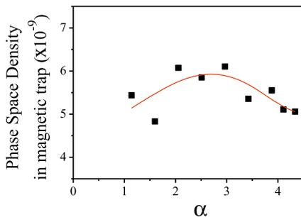
**Figure 4.** Variation in phase-space density of atoms trapped with  $\alpha$ . Continuous curve is for guidance of the eyes.
