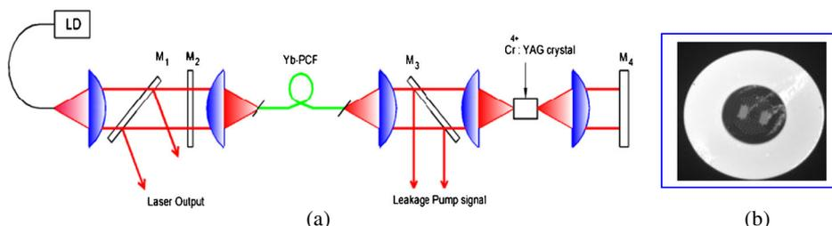
**Figure 1.** (a) Schematic of the passively Q-switched Yb-doped PCF laser, (b) cross-section of PCF.
