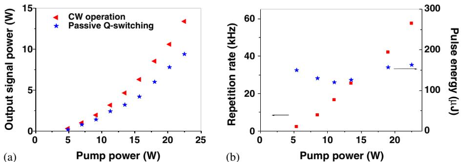
**Figure 2.** (a) Average output power with respect to the launched pump power in CW and passive Q-switching operations. (b) Pulse repetition rate and pulse energy vs. launched pump power.
