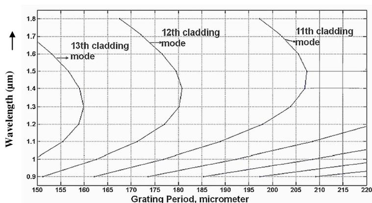
**Figure 2.** Phase matching curves (PMC) for core mode coupling to 11th, 12th and 13th cladding modes in B–Ge co-doped fibre (Fibrecore, UK).
