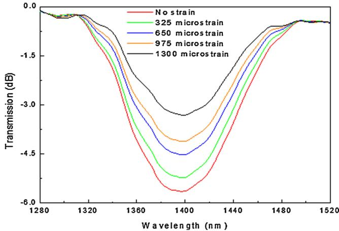
**Figure 3.** Transmission spectrum of the grating corresponding to TAP mode (12th) at different applied longitudinal strain.
