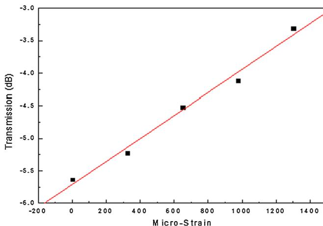
**Figure 4.** Decrease in transmission loss at 1400 nm with increase in longitudinal strain for strain in the range 0–1300  $\mu\epsilon$ .
