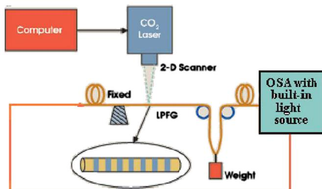
**Figure 1.** Schematic diagram of CO<sub>2</sub> laser-based LPG inscription system.
