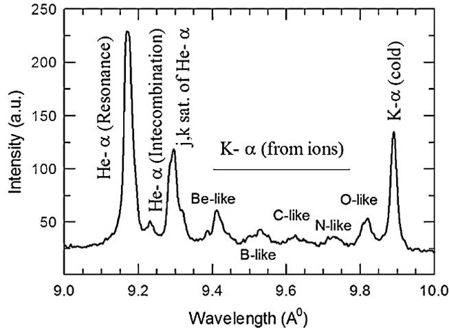
**Figure 1.** Experimental X-ray emission spectrum of the magnesium plasma recorded at an intensity of  $4 \times 10^{17} \text{ W cm}^{-2}$ .
