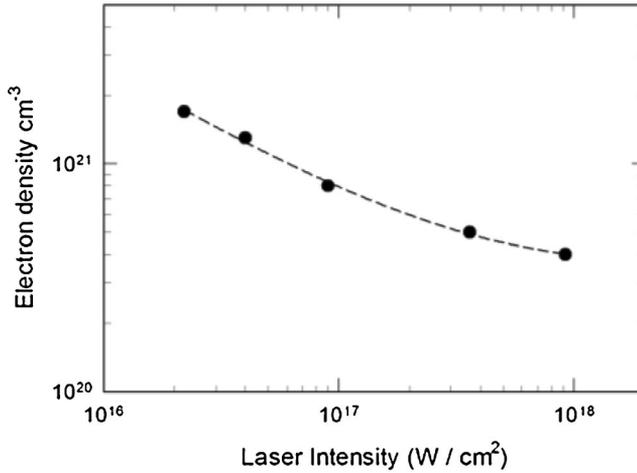
**Figure 3.** Derived electron densities as a function of the laser intensity. The line is drawn to guide the eye.
