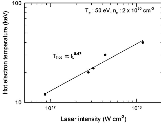
**Figure 5.** Derived hot electron temperature from X-ray line intensity of K- $\alpha$  lines from Be-like ions.
