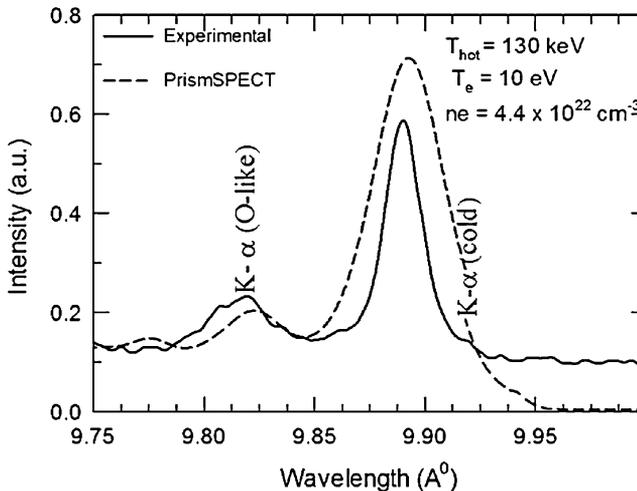
**Figure 4.** Experimental and synthetic spectra of the region around the cold K- $\alpha$  line.
