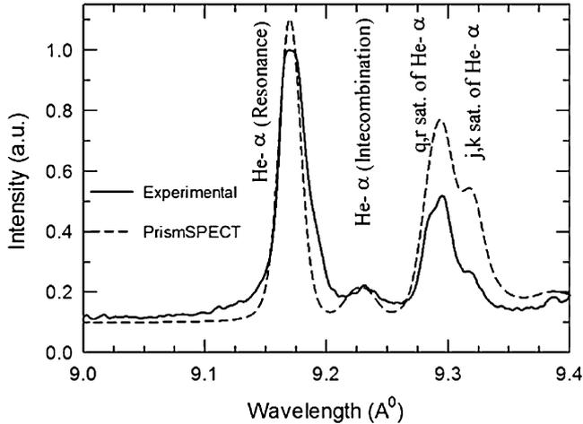
**Figure 2.** Experimental and synthetic spectra of Mg in the region around the He- $\alpha$  resonance line.
