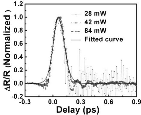
**Figure 6.** Transient reflectivity from QW5 for different pump powers after the removal of slower part.
