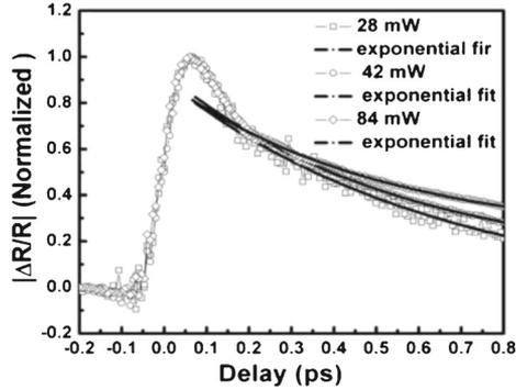
**Figure 4.** Transient reflectivity signal from QW5 for different pump powers, fit to an exponential decay for the latter part of the signal.
