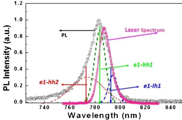
**Figure 2.** Room-temperature cw PL spectrum of QW50 sample along with the femtosecond laser spectrum.
