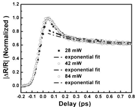
**Figure 3.** Transient reflectivity signal from QW50 for different pump powers, fit to an exponential decay for the latter part of the signal.
