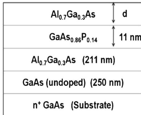
**Figure 1.** QW sample layer structure. For sample QW5  $d=5$  nm and for QW50  $d=50$  nm
