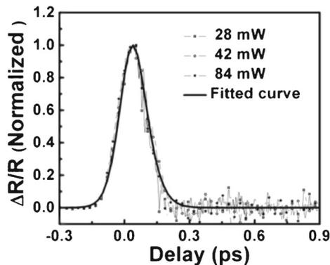
**Figure 5.** Transient reflectivity signal from QW50 for different pump powers after the removal of slower part.
