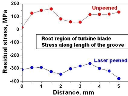
**Figure 3.** Surface profiles of the residual stress on laser-peened and unpeened regions of the root region of the turbine blade.
