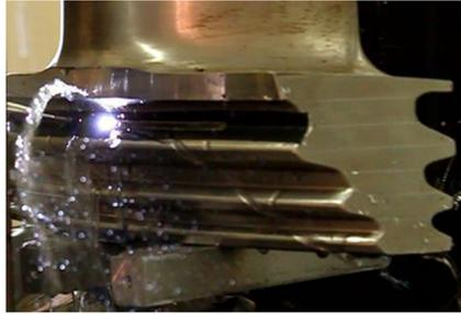
**Figure 1.** LSP of the root of the turbine blade in progress.
