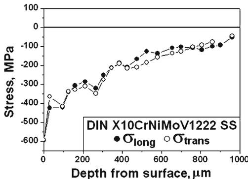
**Figure 4.** Depth profile of residual stresses in laser-peened flat region on the root part of the turbine blade.
