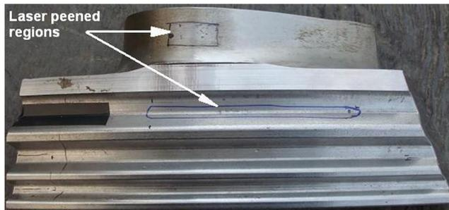
**Figure 2.** Laser-peened regions on the root of the turbine blade.
