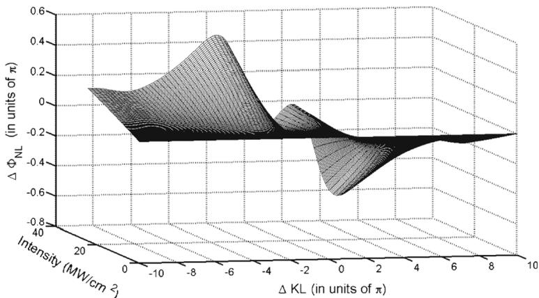
**Figure 4.** Nonlinear phase shift ( $\Delta\Phi_{\text{NL}}$ ) (in units of  $\pi$ ), as a function of crystal phase mismatch,  $\Delta kL$  (in units of  $\pi$ ) and intracavity FW intensity at KTP crystal.
