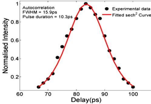
**Figure 3.** Non-collinear SHG intensity autocorrelation trace. Dots: experimental data, continuous line:  $\text{sech}^2$  fit.
