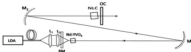
**Figure 1.** Schematic of the soft aperture CSM laser. LDA: laser diode array, L<sub>1</sub> and L<sub>2</sub>: focussing lenses, RM: rear mirror, M<sub>1</sub> and M<sub>2</sub>: folding mirrors, OC: output coupler.
