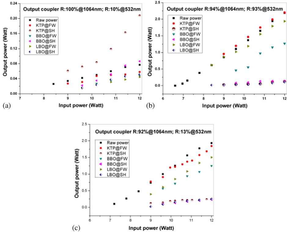
**Figure 2.** Stable mode-locked output power with input pump power for different output couplers: (a) HR@1064 nm and R: 10% @ 532 nm, (b) R: 94% @ 1064 nm and R: 93% @ 532 nm, (c) R: 92% @ 1064 nm and R: 13% @ 532 nm, FW: 1064 nm, SH: 532 nm.
