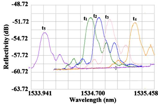
Figure 3. OSA traces showing shift in Bragg wavelength with etching time ( $t_1 < t_2 < t_3 < t_4 < t_5$ ).
