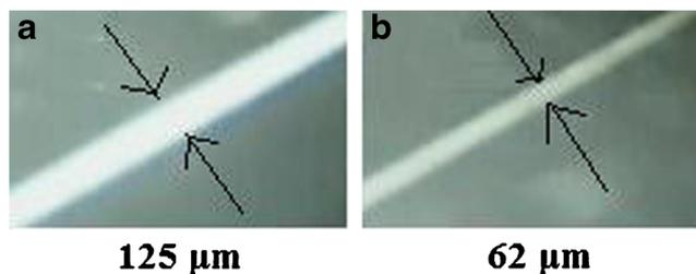
**Figure 2.** Microscopic view of FBG cladding (a) before etching and (b) after etching.
