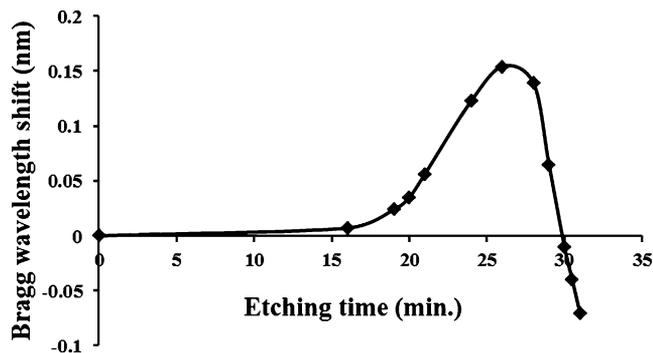
Figure 4. Change in Bragg wavelength as a function of etching time.
