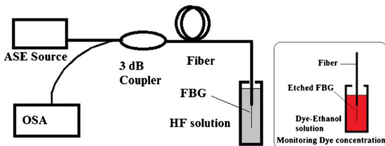
**Figure 1.** Set-up for FBG clad etching/dye concentration monitoring.
