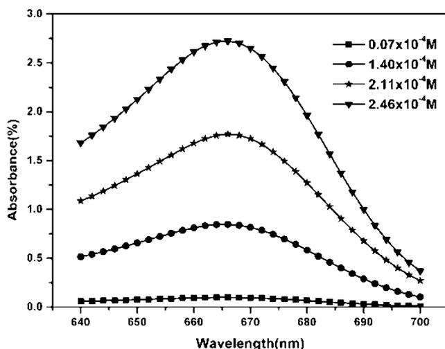
Figure 1. Variation in absorption with dye concentration.
