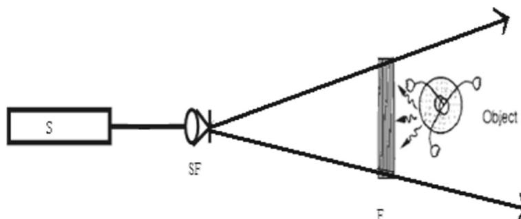
**Figure 5.** Denisyuk configuration for recording reflection holograms.
