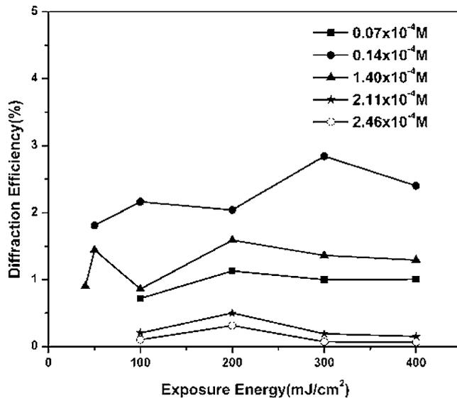
Figure 3. DE vs. exposure energy for an interbeam angle of  $100^\circ$ .
