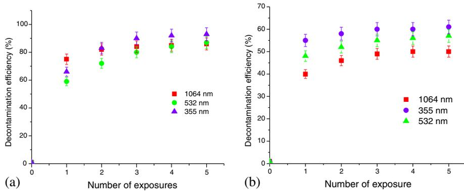
**Figure 3.** Variation of DE as a function of the number of shots. Substrate: (a) Zircaloy, (b) LiF. Contaminant: Milled ThO<sub>2</sub> powder, fluence: 0.2 J/cm<sup>2</sup>.
