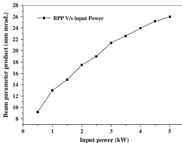
Figure 4. Beam parameter product as a function of power (without aperture).
