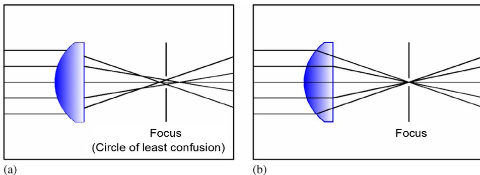
**Figure 1.** Focussing by (a) standard spherical lens and (b) GRADIUM glass lens.
