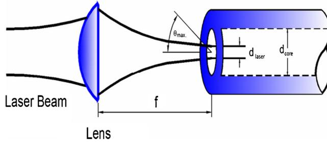
**Figure 2.** A schematic of focussing and launching of laser light into optical fibre.
