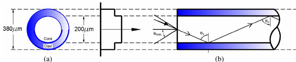
**Figure 3.** A step-index optical fibre. (a) Refractive index profile and (b) total internal reflection at the core-clad interface and numerical aperture.
