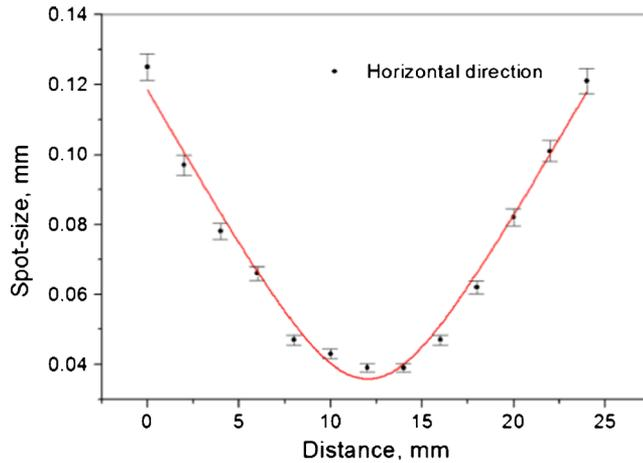
Figure 5.  $M^2$  measured at 1 W output using propagation method.
