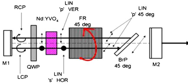
**Figure 2.** Polarization picture of LOPUT cavity.
