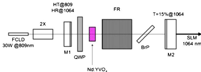
**Figure 1.** Schematic of the LOPUT-based Nd:YVO<sub>4</sub> laser.
