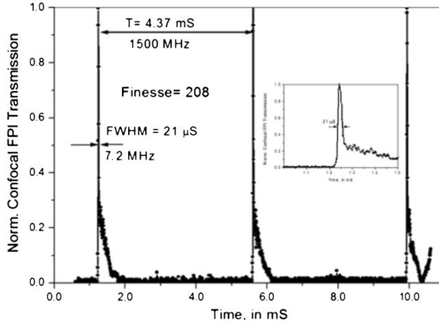
**Figure 4.** SLM performance recorded with a custom-made scanning FPI set-up at 532 nm.
