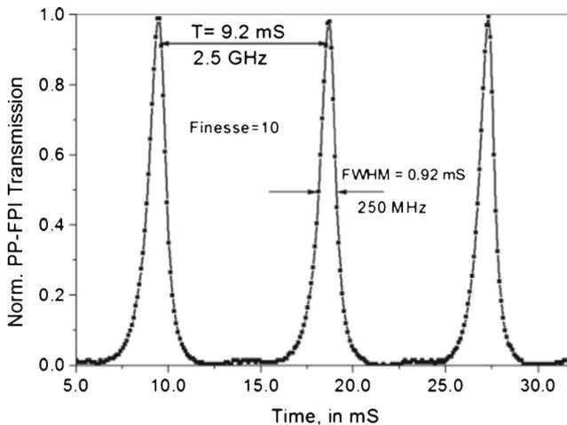
**Figure 3.** SLM Performance recorded with PP-FPI at 1064 nm at 2 W output.
