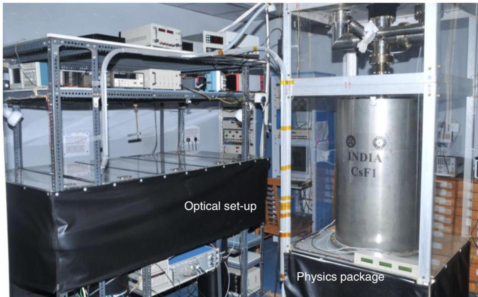
**Figure 1.** Optical set-up and physics package of the cesium fountain clock developed at CSIR-NPL.
