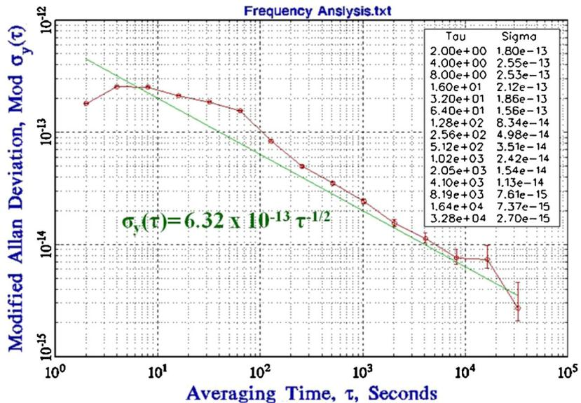
**Figure 3.** Allan deviation of the frequency difference between the fountain and the H-maser as a function of the averaging time.
