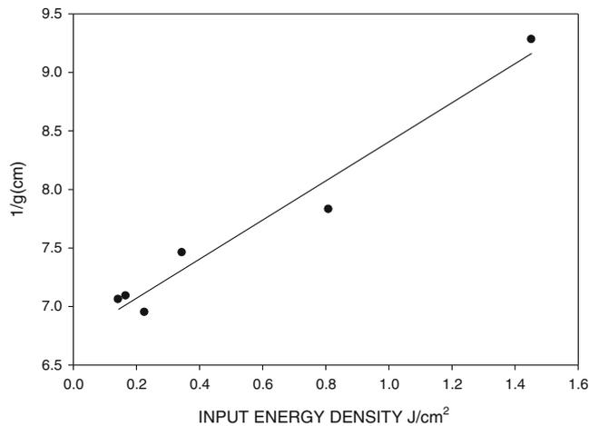
**Figure 3.** Variation of the gain coefficient with input energy fluence.
