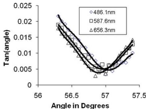
Figure 1. Angle-dependent reflectivity at the three wavelengths for phosphate glass.
