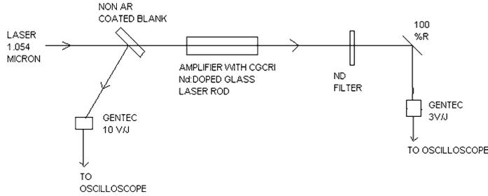
**Figure 2.** Schematic diagram of the gain measurement set-up.
