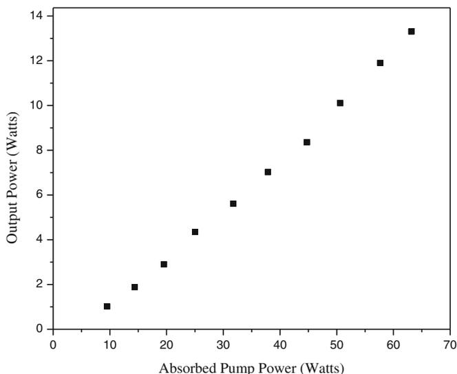
**Figure 2.** Variation of output power vs. input power of EYDFL.
