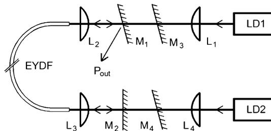
Figure 1. Schematic of the EYDF laser system.
