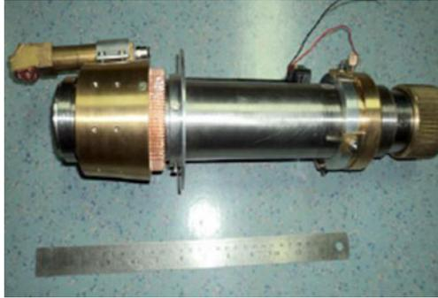
**Figure 6.** Manipulator with laser attachment for welding *in-situ* for repair.
