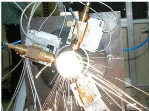
**Figure 4.** A mock-up of laser cutting pressure tubes.
