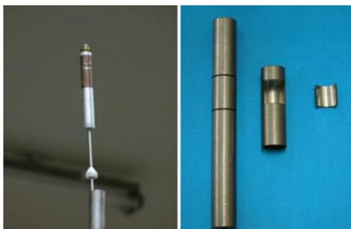
**Figure 5.** A cutting head inserted through the SG tube and the cut sample.
