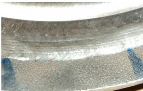
**Figure 9.** View of the end ring from inside after repair by fusing the weld bead.
