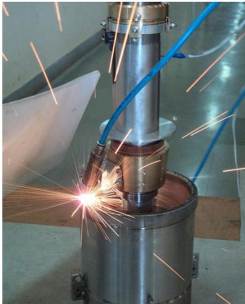
**Figure 7.** Laser cutting in progress to separate the retainer nut sleeve from the upper stand pipe of secondary shut-down system mock-up made at the R&D Centre, Tarapur.
