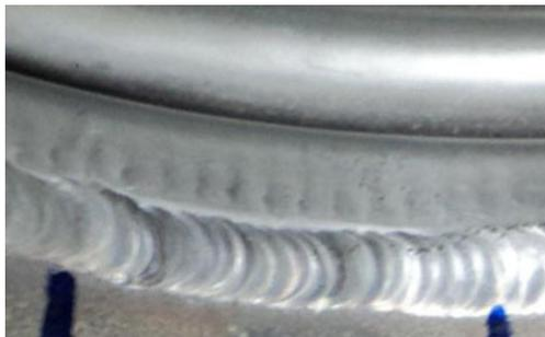
**Figure 8.** View of the end ring weld from inside before repair.
