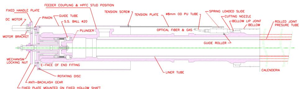
**Figure 2.** A sketch of the bellow lip cutting fixture mounted on the E-face of the coolant channel.
