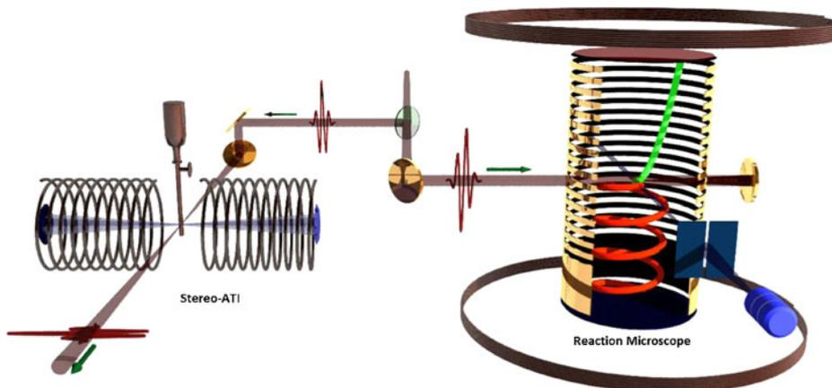
**Figure 1.** Schematic of the experiment. A 6 fs laser pulse is split into two, one part of the beam goes to Stereo-ATI to tag the CEP of the pulse and the other part goes in the reaction microscope and being focussed by a gold mirror to a supersonic gas jet. The ions and electrons formed are detected by the respective detectors. Time-of-flight and position information from the respective detectors are used to reconstruct three-dimensional momentum of electrons and ions in coincidence.
