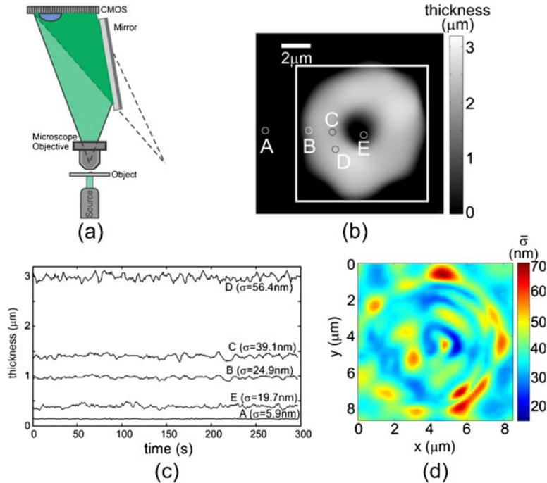
**Figure 4.** (a) Self-referencing DHM using wavefront division geometry, (b) phase contrast image of the analysed RBC, (c) temporal evolution of cell thickness at points shown in (b), (d) mean fluctuation map of the cell. Standard deviations of the fluctuations are also shown.
