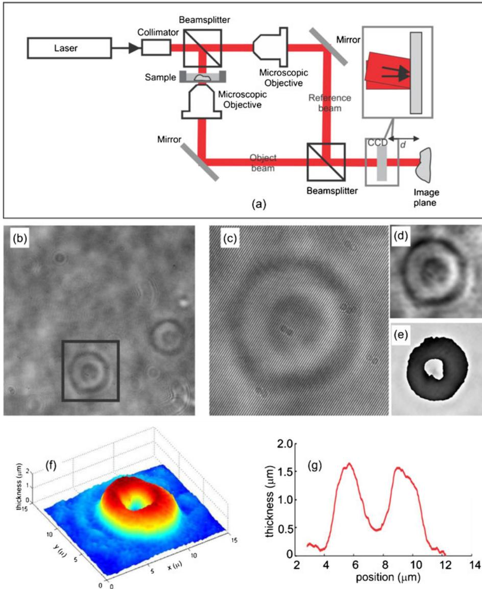
**Figure 1.** (a) Two beam off-axis DHM, (b) recorded hologram, (c) interference pattern inside the marked zone, (d) reconstructed intensity profile, (e) reconstructed phase profile after phase subtraction, (f) thickness profile obtained from the phase using eq. (1), (g) cross-sectional thickness profile of the cell.
