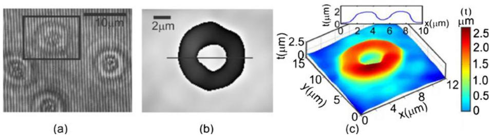
**Figure 3.** Experimental result of imaging RBCs with lateral shearing DHM. (a) Hologram, (b) reconstructed phase of highlighted RBC in (a), (c) 3D rendering of thickness distribution. Inset shows the profile along the line in (b).
