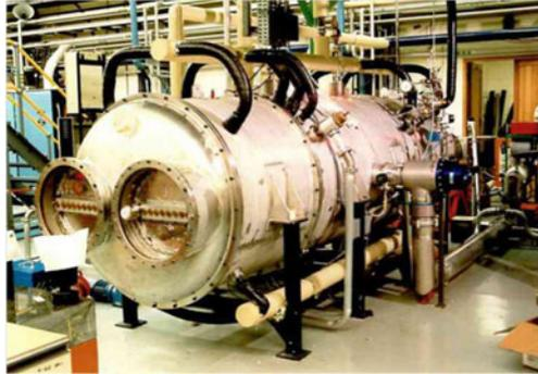
**Figure 7.** Raman cell for stimulated Raman scattering conversion at 2000 Hz.
