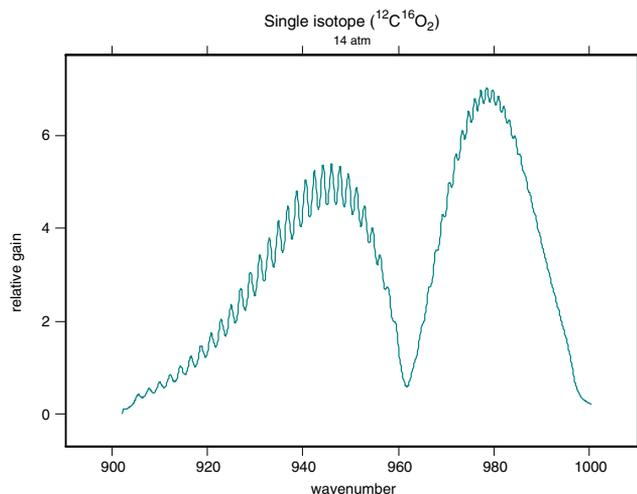
**Figure 3.** Wavelength tunability for CO<sub>2</sub> laser at high pressure.
