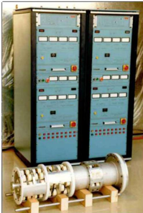
**Figure 5.** Power supply units and four-stage current pulse compressor unit for high laser pulse frequency operation.
