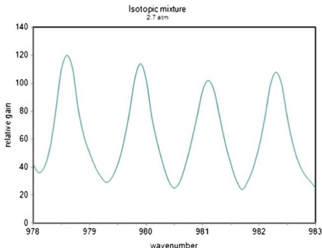
**Figure 4.** Wavelength tunability of isotopic mix CO<sub>2</sub> laser at 2.7 atm.
