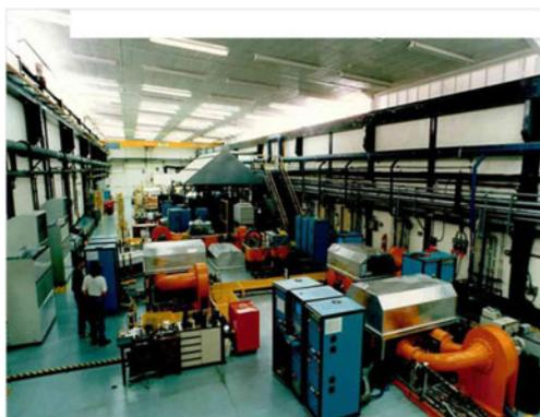
**Figure 6.** Three-wavelength laser chain operating at 2000 Hz for MLIS application.
