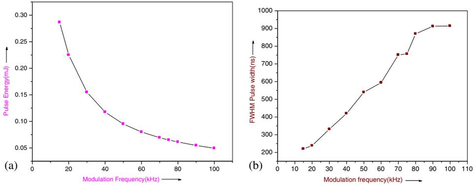
**Figure 10.** (a) Measured pulse energy and (b) measured FWHM pulse width as a function of modulation frequency.
