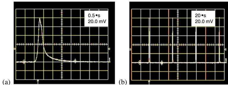
**Figure 11.** Oscilloscope trace of (a) typical AO Q-switched pulse and (b) repetitive occurrence of AO Q-switched pulses at 20 kHz of modulation frequency.
