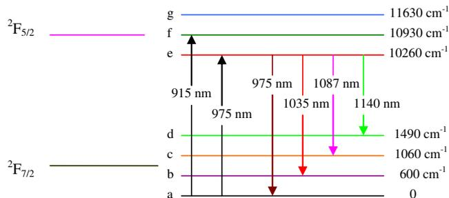
Figure 1. Energy level diagram of Yb ion in silica.
