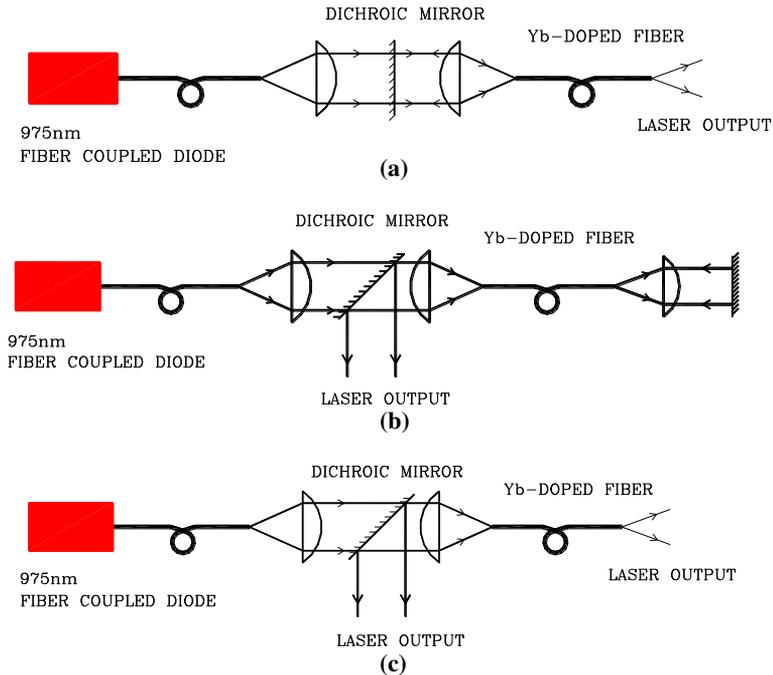
**Figure 4.** (a) High-finesse forward pumping configuration in which output power is taken from the farther end. (b) High-finesse backward pumping configuration in which output power is taken from the pumping end using the tilted dichroic mirror. (c) Low-finesse resonator configuration.
