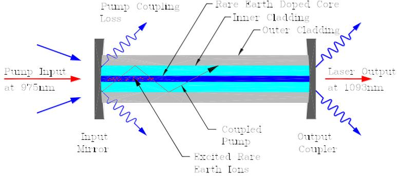
**Figure 3.** Schematic of a double-clad fibre laser configuration.
