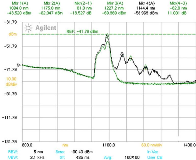
**Figure 6.** Output spectrum in case of low-finesse cavity; the lower trace shows spectrum before the onset of random self-pulsing ( $P_p(0) = 2.5$  W) and the upper trace shows the spectrum after the onset of strong random self-pulsing ( $P_p(0) = 8$  W).
