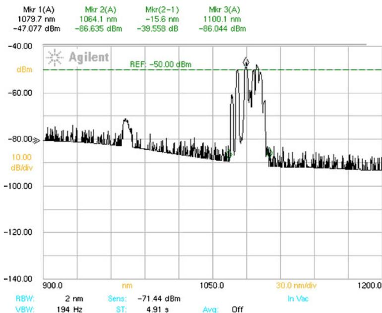
**Figure 8.** Yb-doped CW fibre laser output spectrum at the maximum output power of 165 W.
