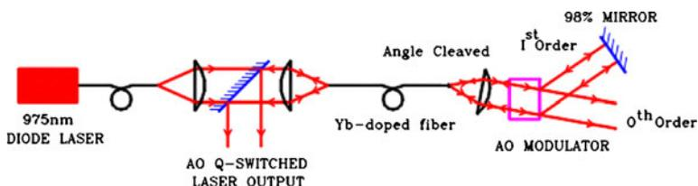
**Figure 9.** Experimental set-up to study Q-switched fibre laser. The dashed line at the fibre end indicates the plane of cleaving of the fibre end at an angle.
