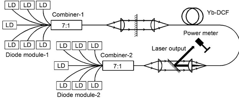
**Figure 7.** A schematic of 165 W Yb-doped CW fibre laser.
