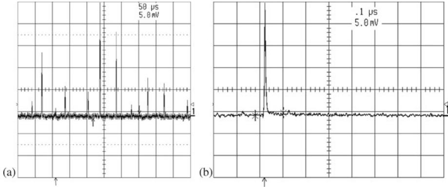
**Figure 5.** (a) Output of the fibre laser, showing random self-pulses in the case of the low-finesse cavity, for an input pump power of 8 W. (b) An expanded oscilloscope trace of one of the random self-pulses.
