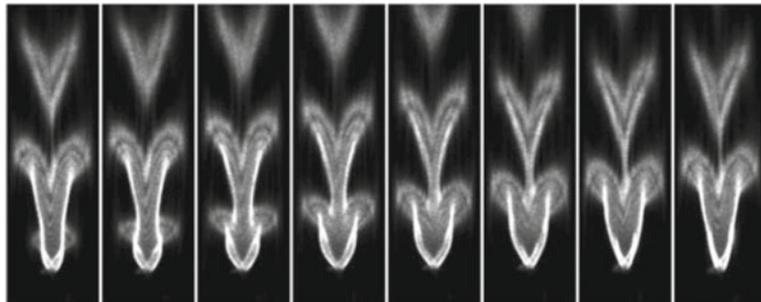
**Figure 3.** Instantaneous schlieren images in the wake of a strongly heated circular cylinder oscillating at 1.5 times the natural frequency of vortex shedding. Main flow is in the vertically upward direction.
