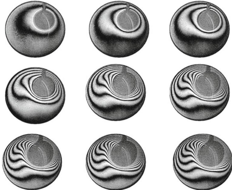
**Figure 2.** Imaging of thermal convection in an eccentric air-filled annulus at selected time instants using a Mach–Zehnder interferometer in the infinite fringe setting.
