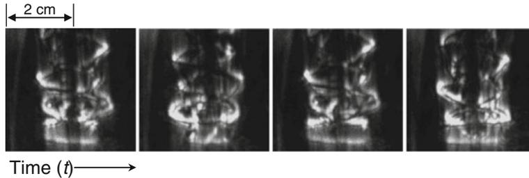
**Figure 4.** Schlieren images of the time-dependent convective field around a KDP crystal growing from its aqueous solution at four different time instants. Bright regions are zones of high concentration gradients. The dark region away from the crystal shows the undisturbed supersaturated solution.
