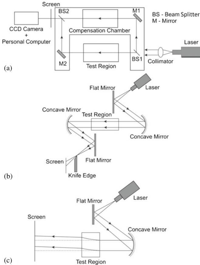
**Figure 1.** Optical configurations of (a) Mach-Zehnder interferometer, (b) laser schlieren, and (c) shadowgraph.
