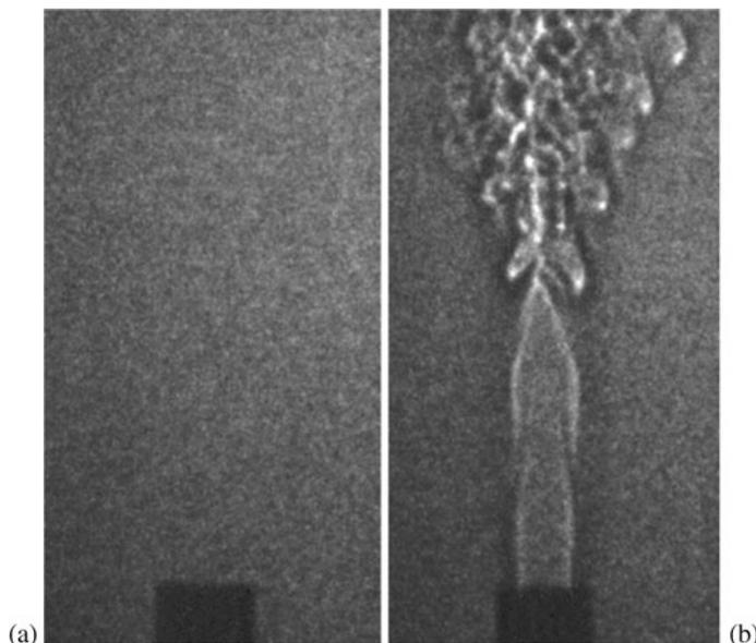
**Figure 5.** Undisturbed screen (a) and light intensity perturbations created in a shadowgraph arrangement (b) when a helium jet is released in the normal atmosphere.
