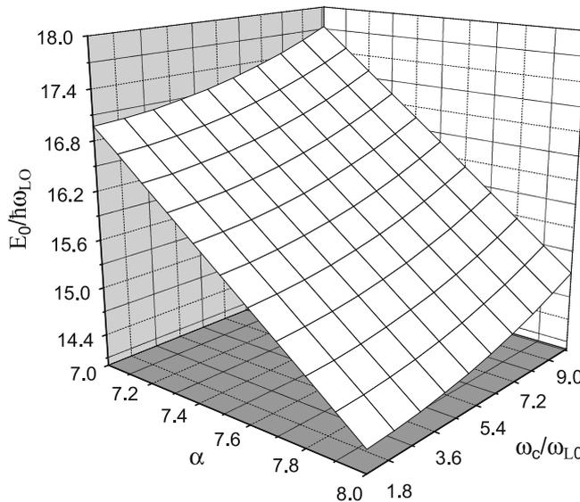
**Figure 1.** The relations of polaron’s ground state energy  $E_0$  with the electron–phonon coupling strength  $\alpha$  and the cyclotron frequency  $\omega_c$  for  $l_1 = 0.35$  and  $l_2 = 0.45$ .
