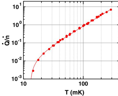
**Figure 4.** Cooling power of CFDR-1200 in the presence of heat load. The solid line is the best fit to the data using Takano’s formula [21] (see text for details).
