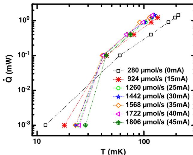
**Figure 2.** The measured cooling power for different flow rates as a function of  $T$ . Numbers in parenthesis indicate the still heater current. An offset of  $1\ \mu\text{W}$  has been included in  $\dot{Q}$  for plotting on log scale.
