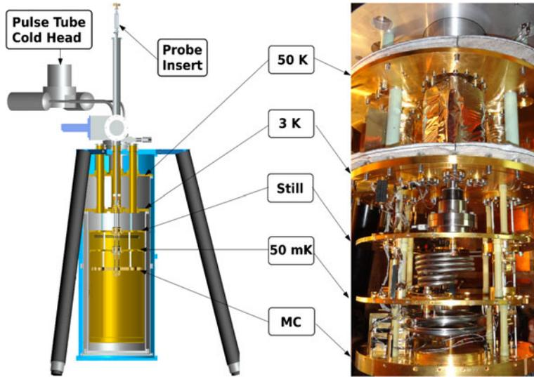
**Figure 1.** Schematics of CFDR-1200 dilution unit at TIFR. The image on the right shows the actual unit.
