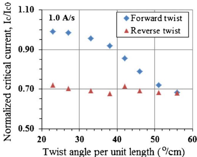
Figure 7. Normalized critical current ( $I_c/I_{c0}$ ) as a function of twist angle per unit length representing the irreversibility of the twisted tape.
