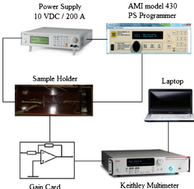
**Figure 4.** Data acquisition schematic for  $I_c$  measurement.
