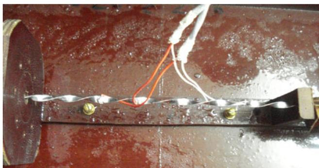
**Figure 3.** Photograph of YBCO tape at  $1530^\circ$  twist angle.
