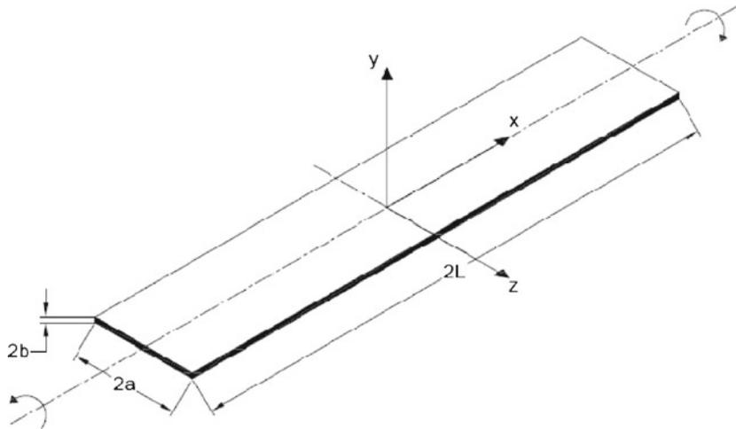
**Figure 1.** Schematic of the YBCO tape.
