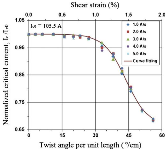
Figure 6. Variation of normalized critical current ( $I_c/I_{c0}$ ) as a function of twist angle per unit length for different ramp rates.
