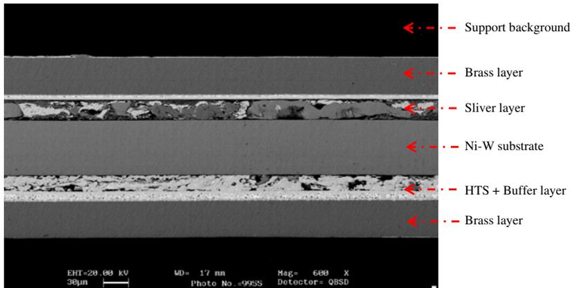
Figure 9. SEM images of the twisted sample showing crack at the interlayer portion of the twisted sample.
