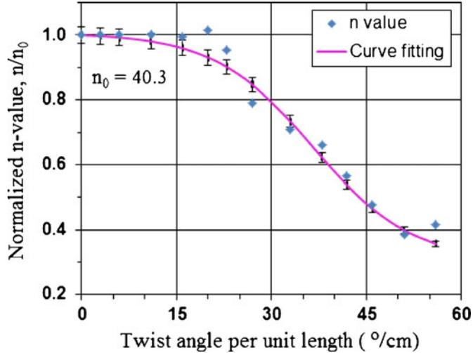
Figure 8. Variation of  $n/n_0$  of YBCO tape as a function of twist angle per unit length.
