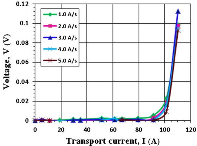
Figure 5. Consolidated  $I$ - $V$  characteristic for  $990^\circ$  twist angle for various ramp rates.
