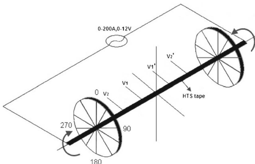
**Figure 2.** Experimental set-up for  $I_c$  measurement under twisting.
