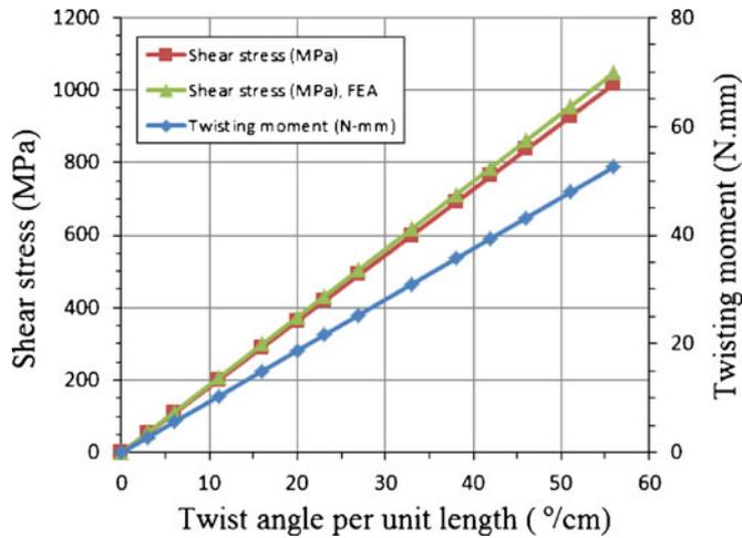
**Figure 10.** Variation of the shear stress and twisting moment as a function of twist angle per unit length.
