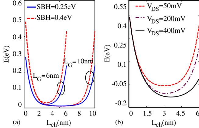
**Figure 2.** (a) Energy of the first subband along the channel for  $SBH=0.25\text{ eV}$  and  $0.4\text{ eV}$  as the gate length scales down from  $10\text{ nm}$  to  $6\text{ nm}$  at  $V_{DS} = 50\text{ mV}$ ,  $V_{GS} = 0.45\text{ V}$ . (b) Impact of drain voltage on the curvature of the lowest subband for  $SBH=0.4\text{ eV}$ ,  $L_G = 6\text{ nm}$  and  $V_{GS} = 0.45\text{ V}$ . As the drain voltage increases, the curvature of the subband is smoothed out.
