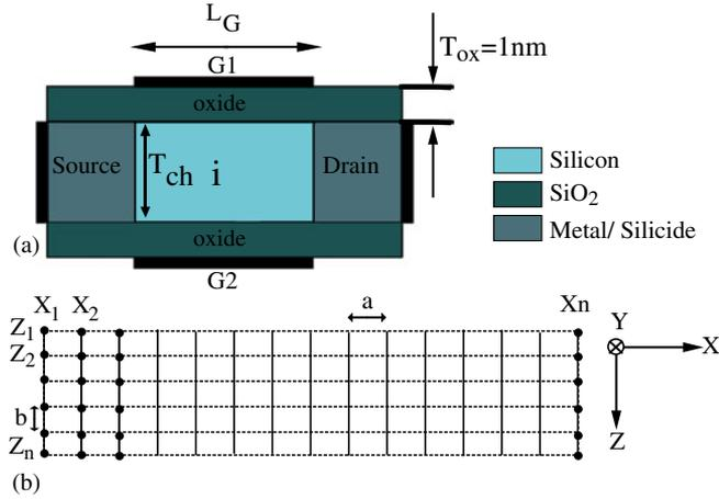
**Figure 1.** (a) Double gate SOI MOSFET with metal source/drain simulated in this study. (b) 1D Schrödinger equation is solved in each slice in depth of the channel at each grid in the transport direction.
