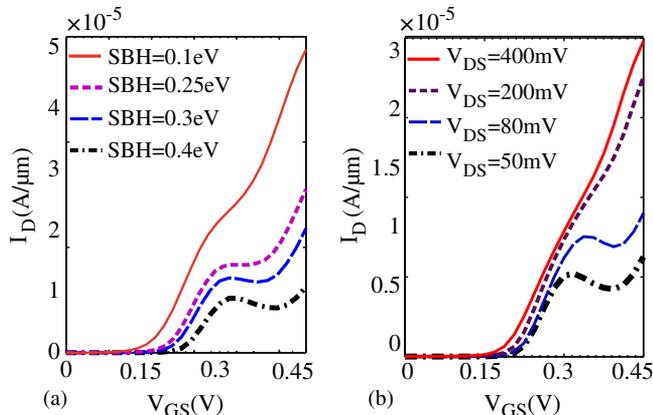
**Figure 5.** (a) Impact of SBH on the transfer characteristic of SBMOSFET for  $L_G = 6$  nm,  $V_{DS} = 50$  mV and  $T = 77$  K. For high effective SBHs resonant tunnelling occurs. (b) Impact of drain voltage for SBH = 0.4 eV,  $V_{GS} = 0.45$  V and  $L_G = 6$  nm. As  $V_{DS}$  increases, the curvature of the channel is diminished and resonant tunnelling is gradually suppressed.
