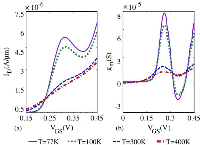
**Figure 4.** (a)  $I_D$ - $V_{GS}$  characteristic of SBMOSFET and (b) transconductance ( $g_m$ ) vs. gate voltage for  $V_{DS} = 50$  mV,  $V_{GS} = 0.45$  V,  $L_G = 6$  nm and SBH = 0.4 eV as the temperature varies from 77 K to 400 K. Negative differential resistance is apparent for low temperatures.
