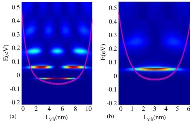
**Figure 3.** Local electron density of states (LDOS) and first subband profile along the channel at  $V_{GS} = 0.45$  V,  $V_{DS} = 50$  mV, SBH = 0.4 eV for (a)  $L_G = 10$  nm and (b)  $L_G = 6$  nm. As  $L_G$  scales down to 6 nm, the energy separation between resonance states increases. Bright regions indicate higher density of states whereas dark blue regions indicate lower density of states.
