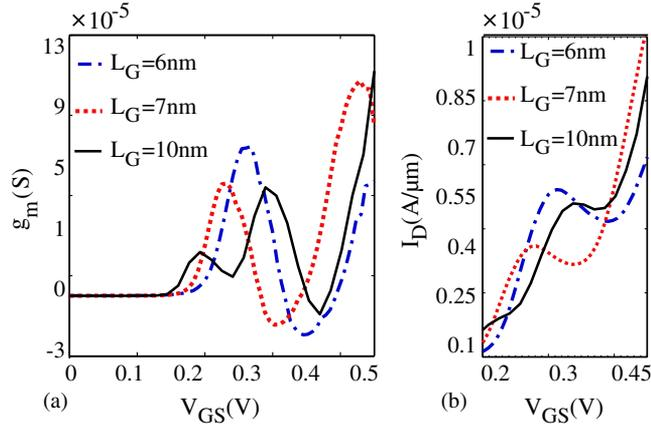
**Figure 6.** (a) Transconductance ( $g_m$ ) vs. gate voltage and (b)  $I_D$ – $V_{GS}$  characteristic of SBMOSFET for  $V_{DS} = 50$  mV,  $V_{GS} = 0.45$  V,  $SBH = 0.4$  eV and  $T = 77$  K as the channel length scales down from 10 nm to 6 nm. The first resonant tunnelling occurs at higher gate voltages as  $L_G$  scales down to 6 nm.
